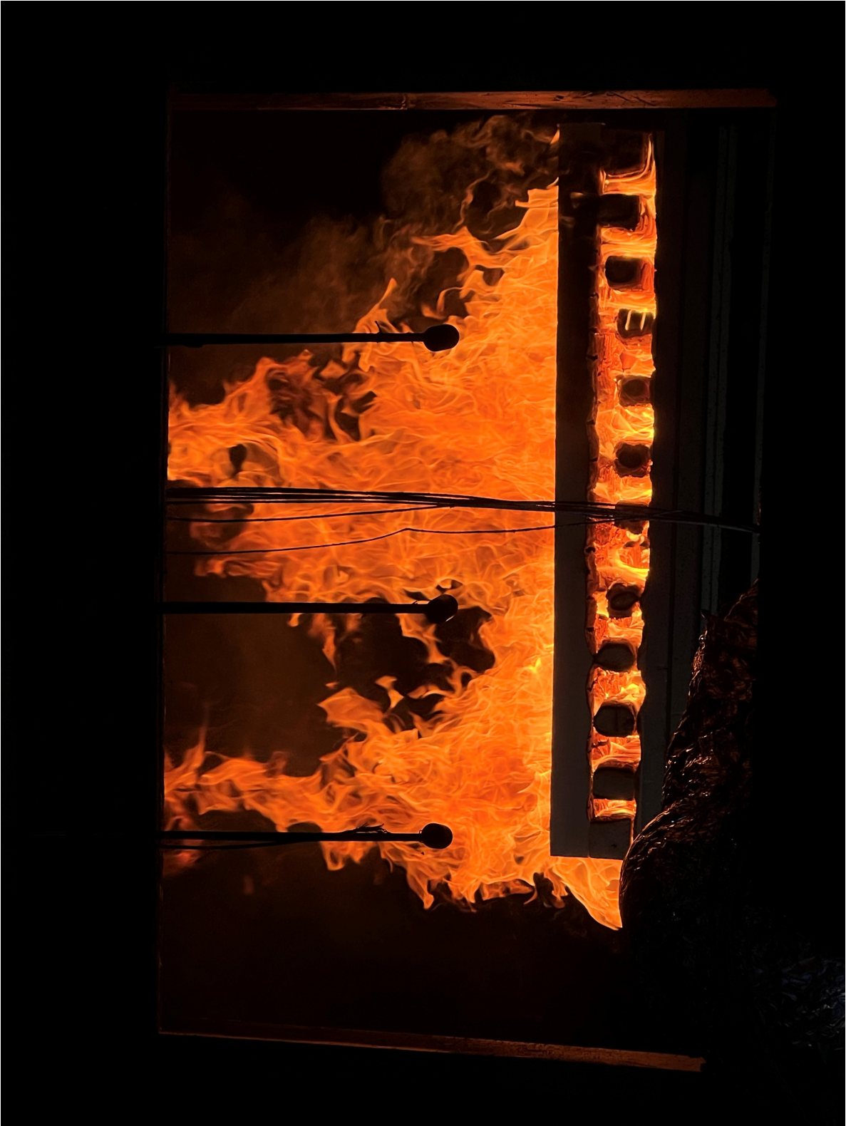
Figure A.5: A photograph of the timber crib burning in an ISO room with the larger opening. Photograph taken after approximately 1900 seconds.
