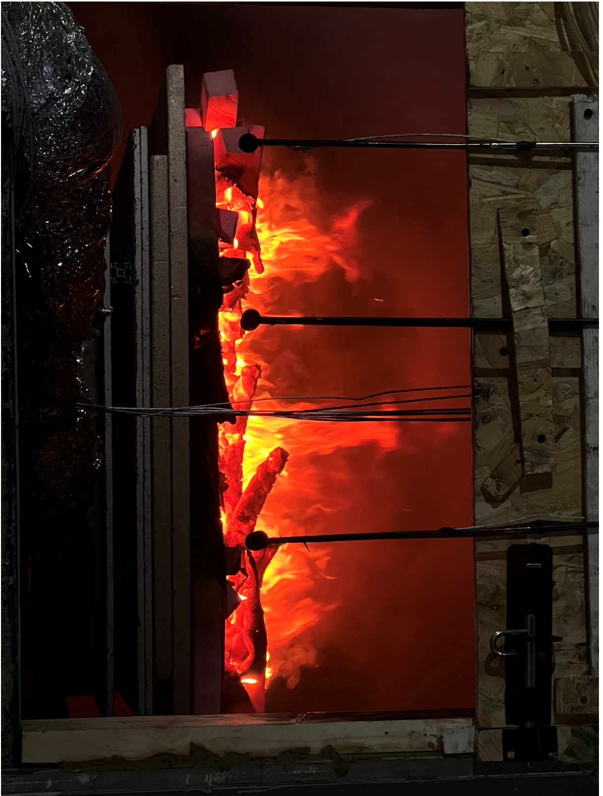
Figure A.4: A photograph of the phenolic foam crib burning in an ISO room with the larger opening. Photograph taken after approximately 700 seconds.
