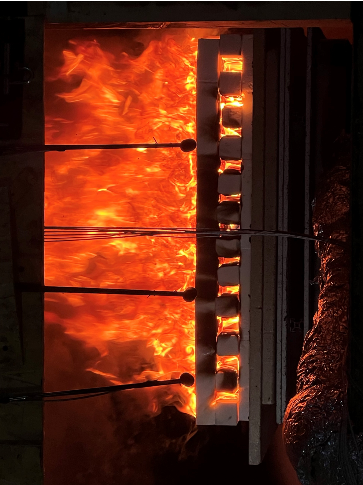
Figure A.3: A photograph of the PIR crib burning in an ISO room with the larger opening. Photograph taken after approximately 100 seconds.
