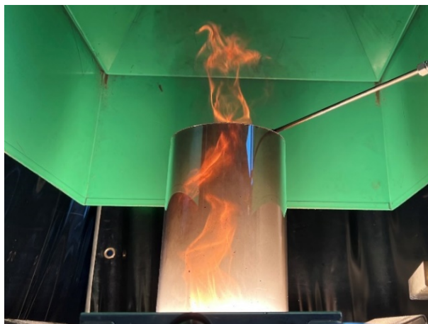
Figure 4.2: The oxidation of species beyond the quartz tube in the FPA. Such external flames are often uncontrollable and suggest that the effluent comprises of a significant proportion of unburnt species.
