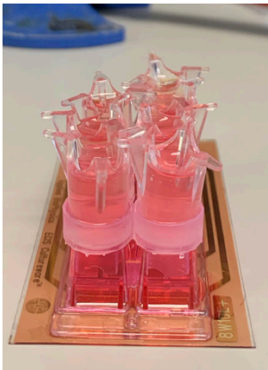
Figure 5.5. Transwell setup on ECIS, showing inserts into 3d-printed connectors, further introduced into an ECIS plate well.
