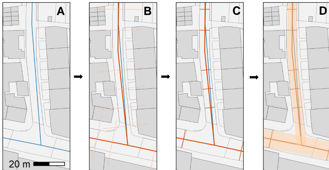
Figure 4.2 Example of modelled road geometry modification and width assignment strategy. See section ‘Road network’ for a detailed description. ©Crown copyright/MasterMap 2021. Ordnance Survey/Edina supplied service.
