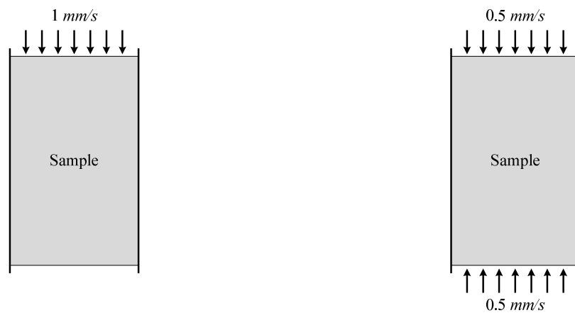
(a) Unrestraint geometries (Experimental)
