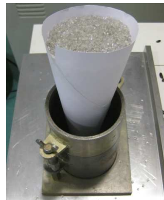
(c) Ascending cone with no impact filling method
