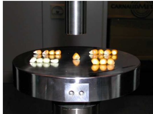
(b) Rigid compression platen combined with 3D laser scan of surface profile
