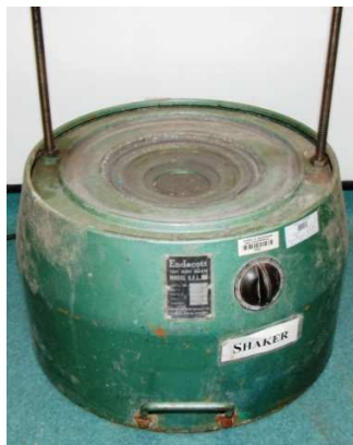
(b) Vibrating 'shaker' device to produce denser packing
