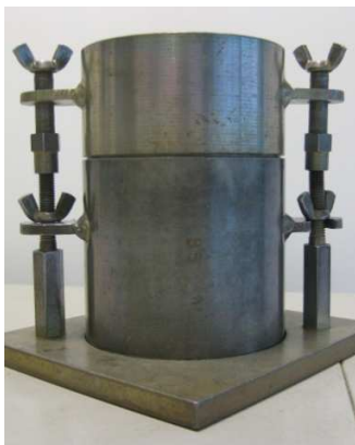
(a) BSI 1 l compaction mould with top ring for aiding filling
