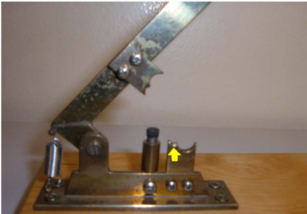
Figure 2.1 A (Top). A custom designed apparatus which can be operated by one person. The dimensions are 30cm long and 12 cm wide at the base and 7 cm high. Figure 2.1 B (Bottom). The tibia is placed across the fulcrum at the point marked by the arrow. The 2 braces on the upper part of the apparatus swing down with the lever handle and break the tibia over the fulcrum.
