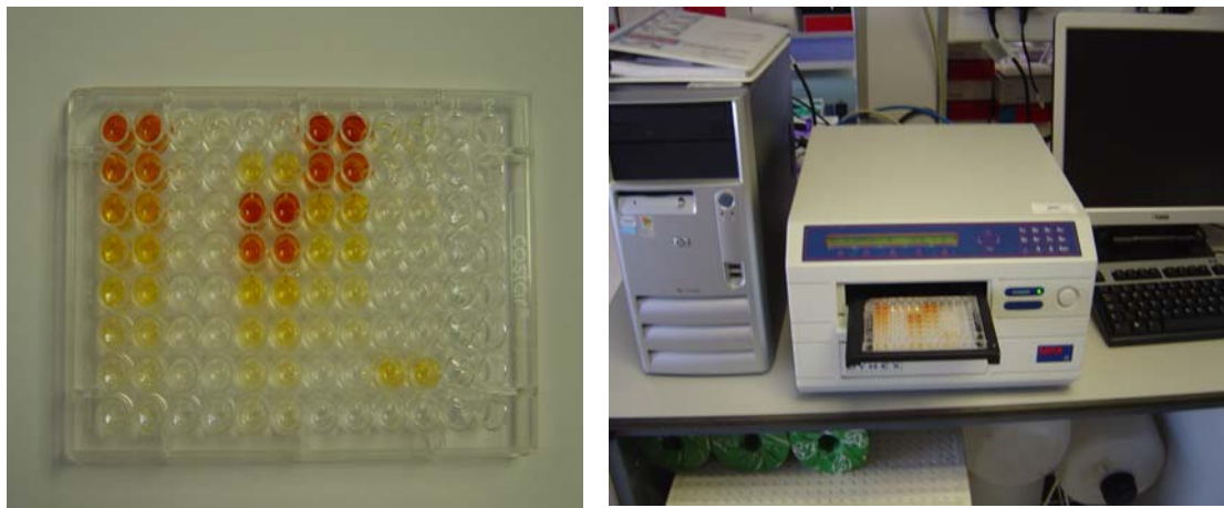
Figure 5.2 A microtitre plate (left) and the optical density measuring equipment (right).
