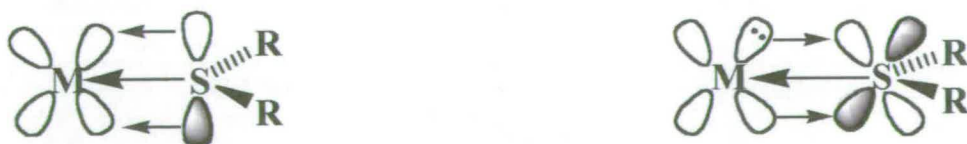
Figure 1.7 Metal-thioether bonding assuming sp^2 hybridisation at sulfur
