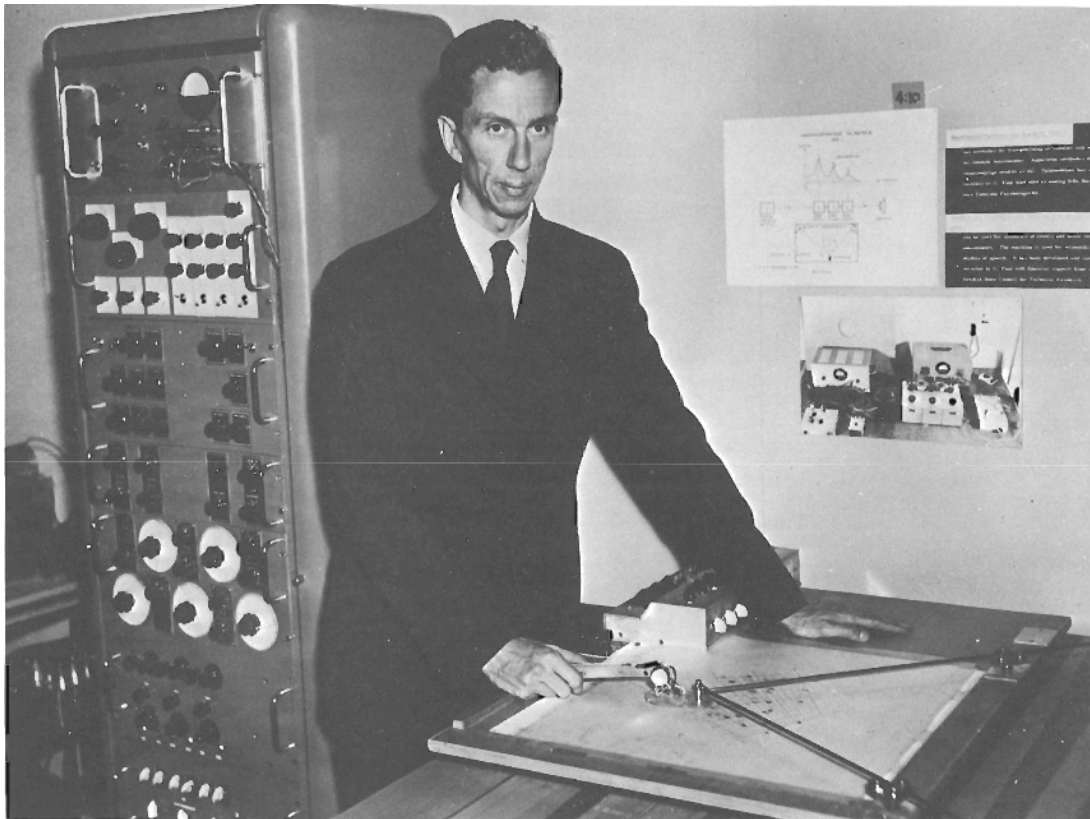
Figure 2.2: Gunnar Fant demonstrates his OVE I synthesiser. A mechanical arm was employed to actively plot out the first two formant frequencies. Image is taken from Watanabe et al. (1979) , original photographer unknown.
