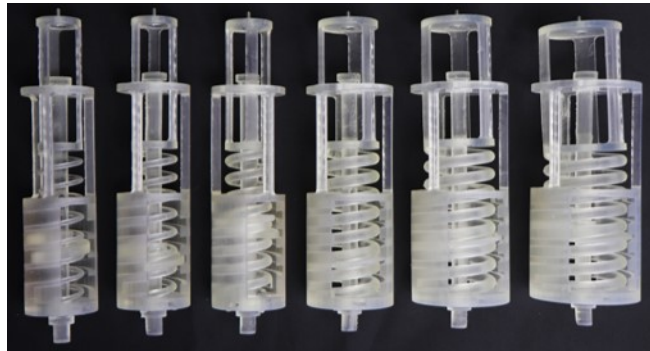
Figure 3.6: From left to right: VSMs in configurations 1 to 6 (Table 3.1) after supports removal, IPA cleaning and additional curing in UV chamber.
