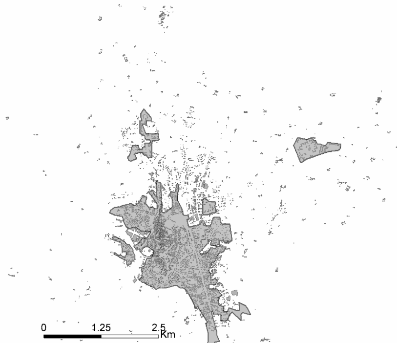
Figure 12b: IGN France settlement boundaries at 1:250 000 with input buildings selected from IGN BDTopo® dataset.
