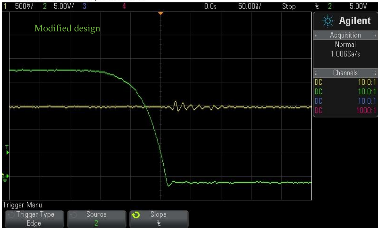
Figure 2.70. Half-bridge negative transients and ringing test at MOSFET turn-on. Top - original design, bottom – modified design by decreasing the slew rate by two times and replacing 0.01 \mu F bridge decoupling capacitor by 1 \mu F. Yellow trace – load current, green trace – MOSFET drain-to-source voltage (MOSFET current is about 10 A).
