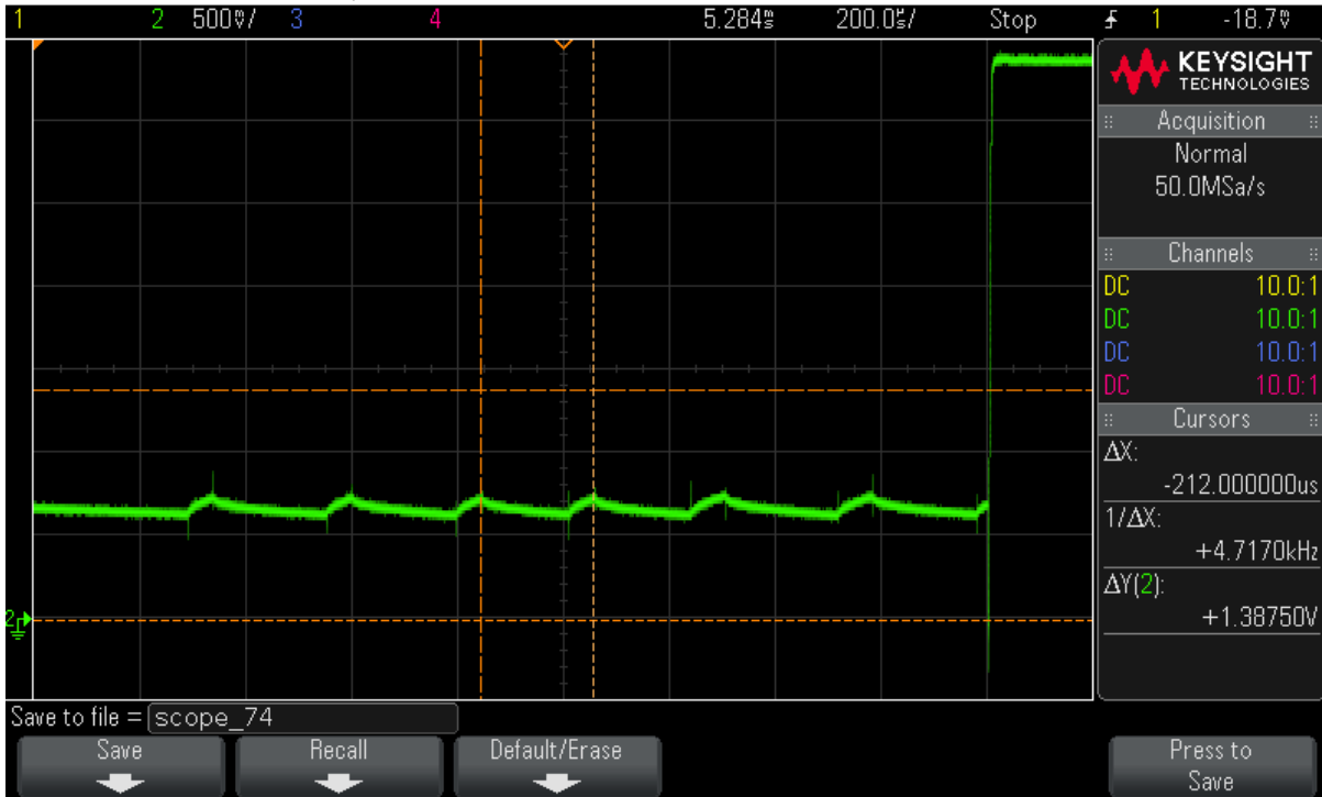
Figure 2.63. PWM frequency measurement at the hold phase of the coil current profile.
