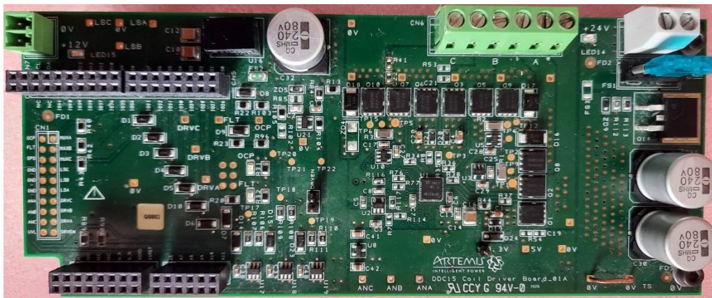
Figure 2.50. Photograph of the next-generation coil driver (NGCD) prototype board.
