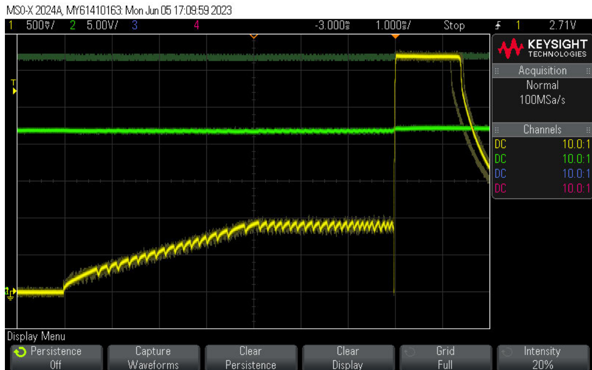
Figure 6.19. Coil current profile at the sweep in firing angle test with the valve response time stabilisation (RTS) enabled. DDP150S pumping cycle.
