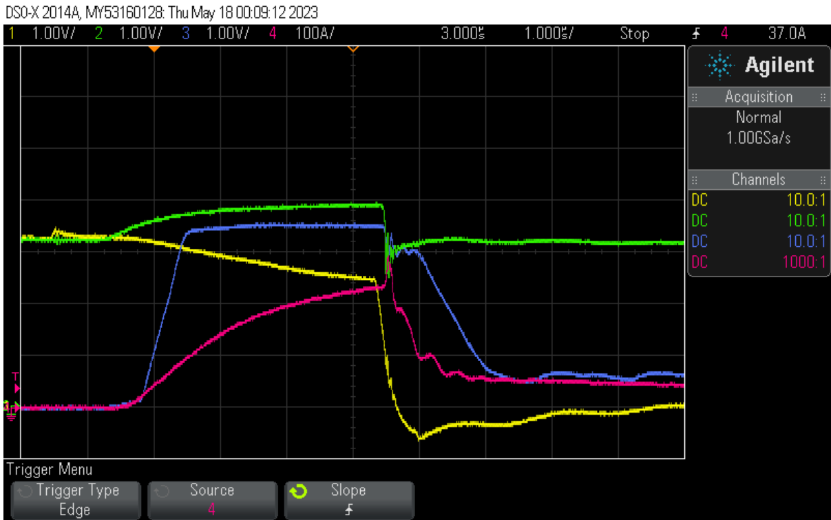
Figure 2.53. Short-to-supply test (Low-side OCP). Yellow waveform – DRV_ENABLE pin voltage, red waveform – short circuit current, green waveform – nFAULT pin voltage, blue waveform – CSA output voltage.
