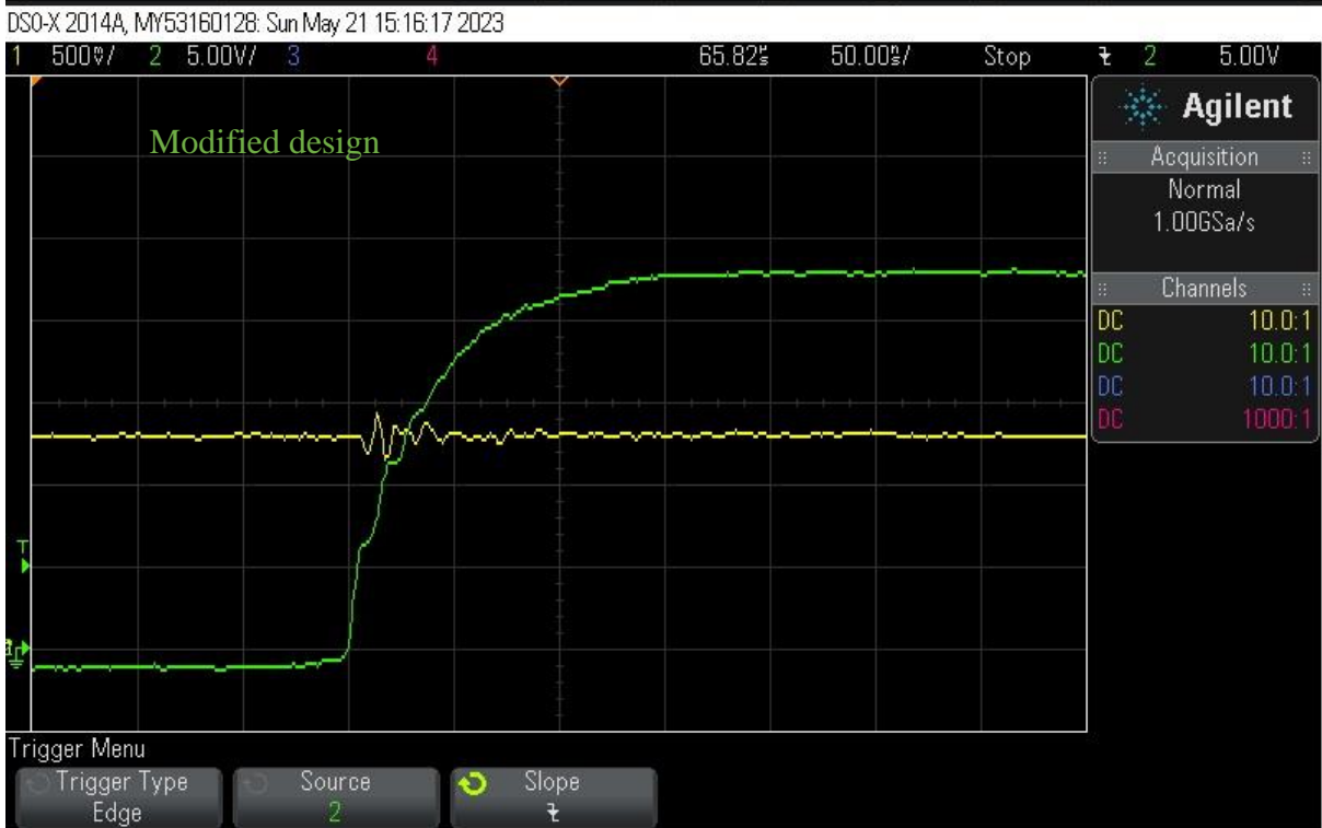
Figure 2.69. Half-bridge negative transients and ringing test at MOSFET turn-off. Top - original design, bottom – modified design by decreasing the slew rate by two times and replacing 0.01 \mu F bridge decoupling capacitor by 1 \mu F. Yellow trace – load current, green trace – MOSFET drain-to-source voltage (MOSFET current is about 10 A).
