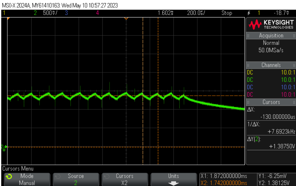
Figure 2.62. PWM frequency measurement at the peak phase of the coil current profile.
