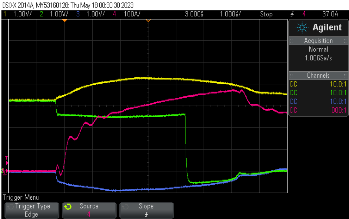
Figure 2.51. Short-to- GND test (DRV8320H OCP). Yellow waveform – DRV_ENABLE pin voltage, red waveform – short circuit current, green waveform – nFAULT pin voltage, blue waveform – CSA output voltage.
