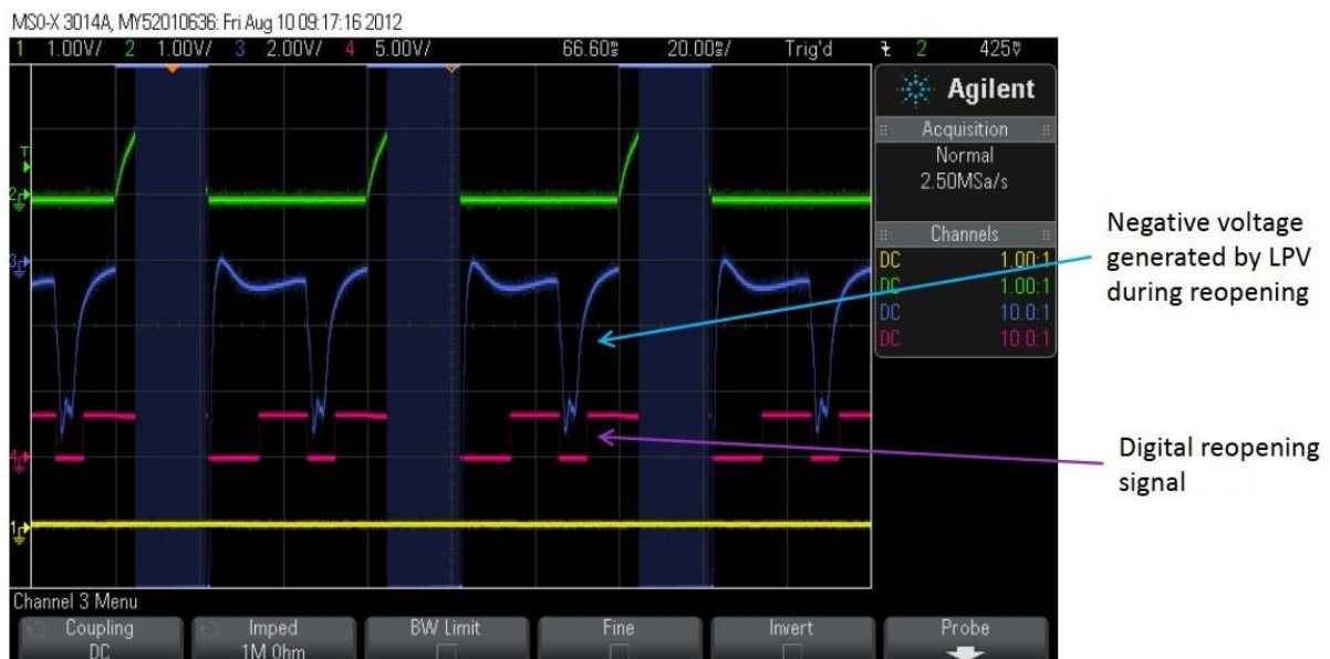
Figure 3.4. Test results of the back-EMF detection circuit that is proposed in the patent (The figure is taken from [60]).
