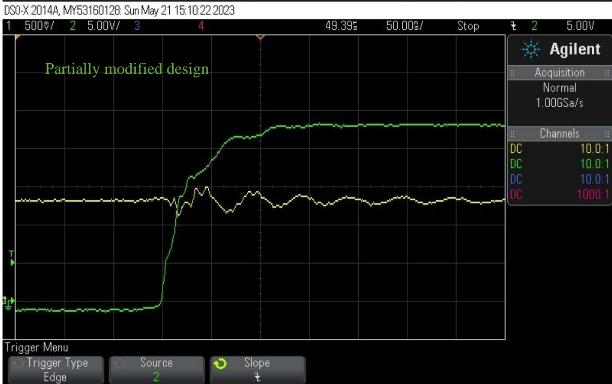
Figure 2.67. Half-bridge negative transients and ringing test at MOSFET turn-off. Top - original design, bottom - partially modified design by decreasing the slew rate by two times. Yellow trace – load current, green trace – MOSFET drain-to-source voltage (MOSFET current is about 10 A).
