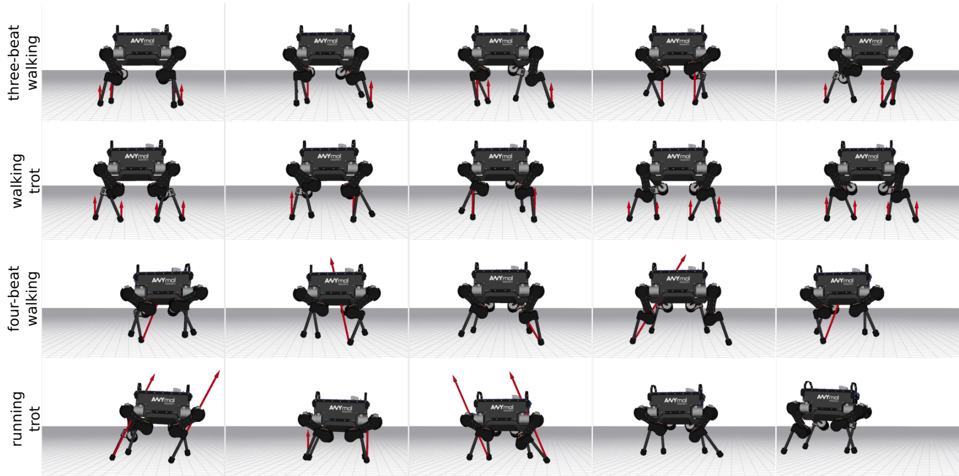
Figure 49: Snapshots of different gait pattern discovered for 3D quadruped robot ANYmal: three-beat walking (Gait 1), walking trot (Gait 2), four-beat walking (Gait 5) and running trot (Gait 6). Red arrows represent contact force vectors.
