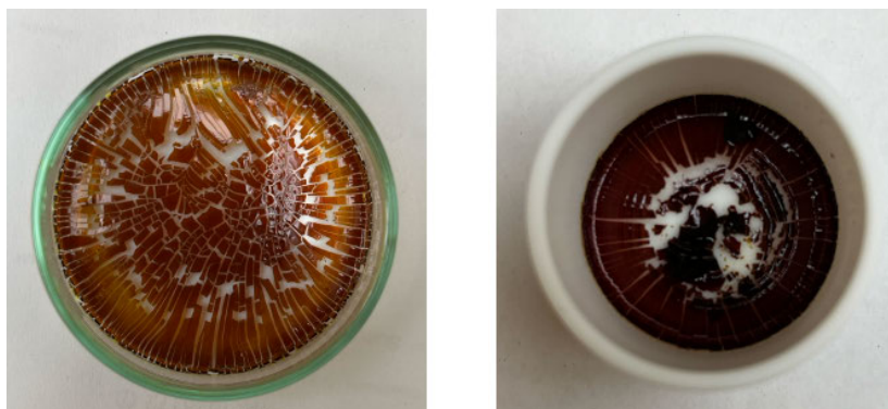
Figure 5.3a: Membrane casted from SBL-PIM (left) and SBL-AO-PIM (right) with DMSO
