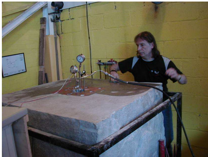
Figure 4.14: Magnetostrictive source clamped in the granite block.
