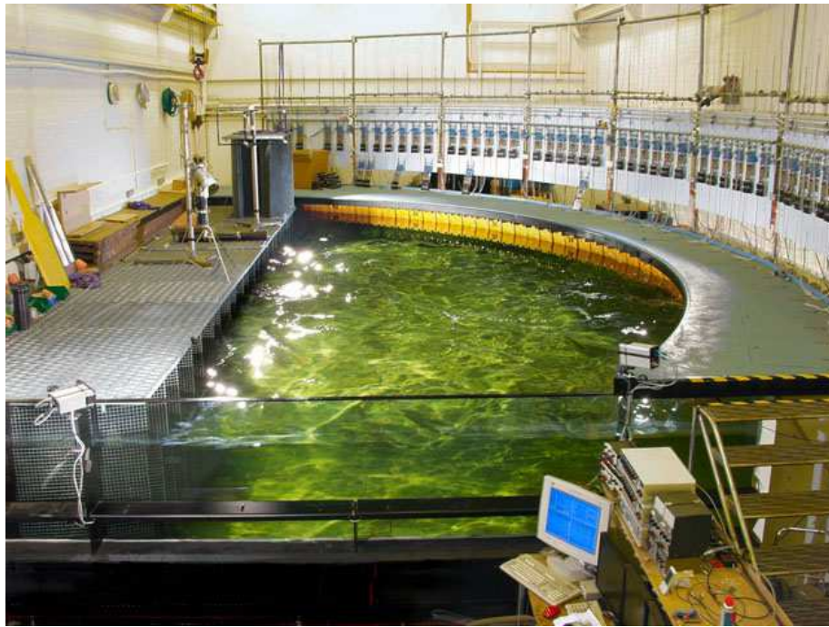
Figure 4.12: Photograph of the wave-tank used for the fluid-filled tube testing.
