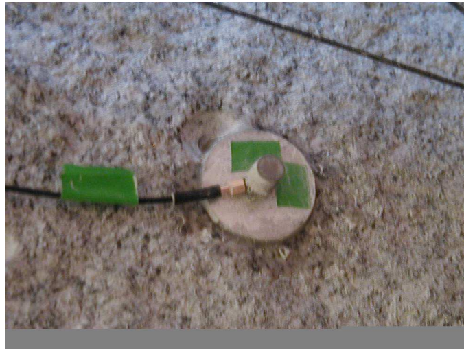
Figure 4.15: One of the accelerometers fixed into the block.
