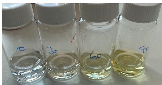
Figure 6.2 Ceftazidime in water upon exposure to UVC irradiation for (left to right) 0, 30, 60 and 90 minutes
