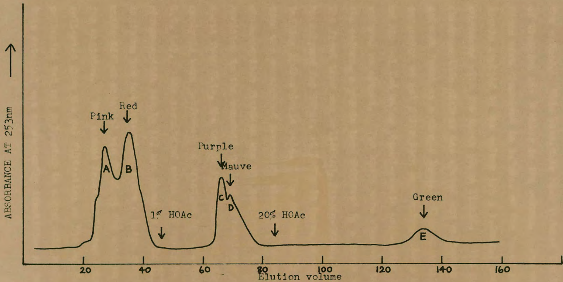
FIG.10. Absorption trace (at 253nm) of chromopeptides eluted from Bio Gel P-6 column.
