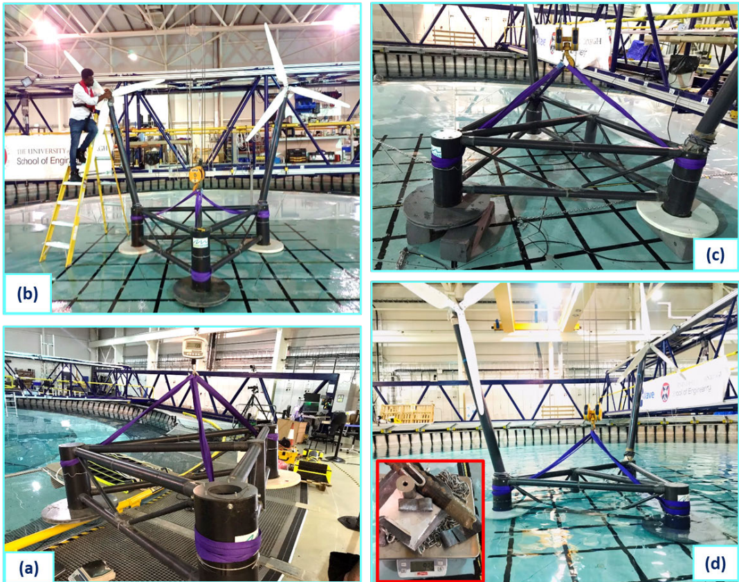
Figure A.3: Artistic depictions illustrating the assembly and configuration of the floating system. Proceeding clockwise from the bottom left: (a) depiction of the W2Power hull being transit via crane, (b) assembled towers with turbines being affixed, (c) attachment of mooring lines to fairleads under the bow column, (d) the assembled model floating with the crane partially released, accompanied by ballasting using mass pieces on the scaler (small photo outlined in red).
