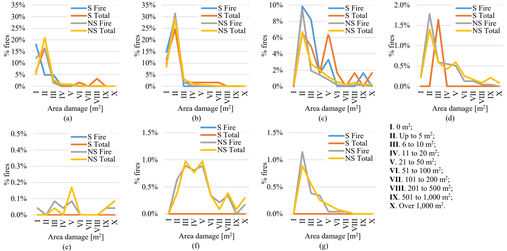
a. No fire damage; b. Limited to item ignited; c. Limited to room of origin; d. Limited to floor of origin; e. Limited to two floors; f. Whole building/ more than two floors; g. Roofs/Roof spaces; S. Sprinklers; NS. No Sprinklers; Fire. Fire damage; Total. Total damage
