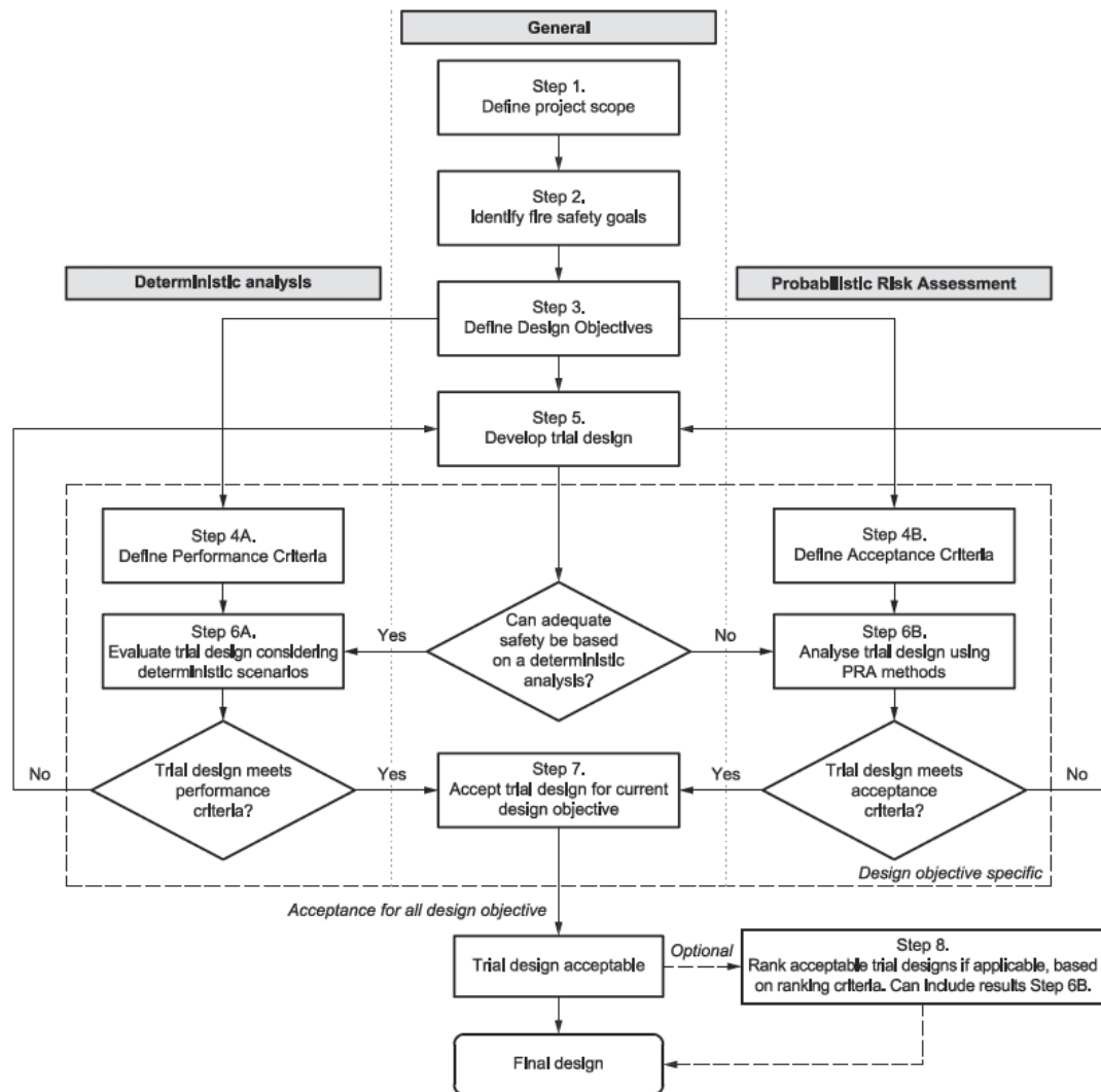
Figure 27: Flow chart to demonstrate adequate safety (BSI PD 7974-7, 2019)
