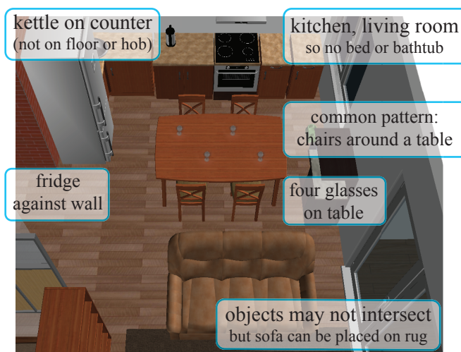
Figure 4.2: An example room, showing various constraints and relations that a model over layouts must capture. The layout and CAD models are from the SUNCG dataset (Song et al., 2017)
