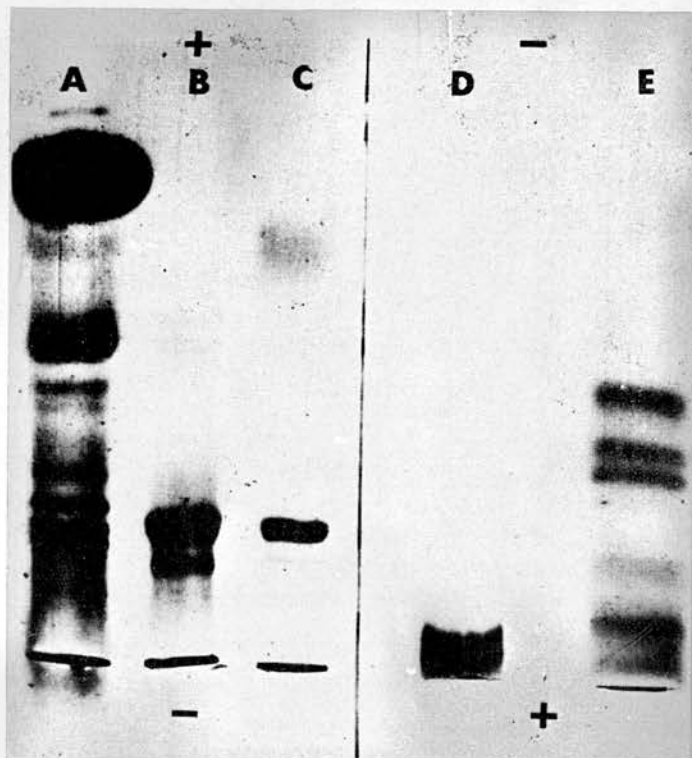
Fig. 1. Starch-gel electrophoresis of human serum \alpha_2 -macroglobulin after papain digestion. A, B and C. Horizontal starch-gel electrophoresis using the discontinuous buffer system of POULIK 6 . A, whole human serum; B, intact \alpha_2 -macroglobulin; C, papain-digested \alpha_2 -macroglobulin. D and E. Horizontal starch-gel electrophoresis in 8 M urea and formate buffer 1 . D, intact \alpha_2 -macroglobulin; E, papain-digested \alpha_2 -macroglobulin. In both cases electrophoresis was conducted at 20 V/cm for 6 h.
