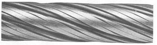
Lang's Lay Rope. Worn.
