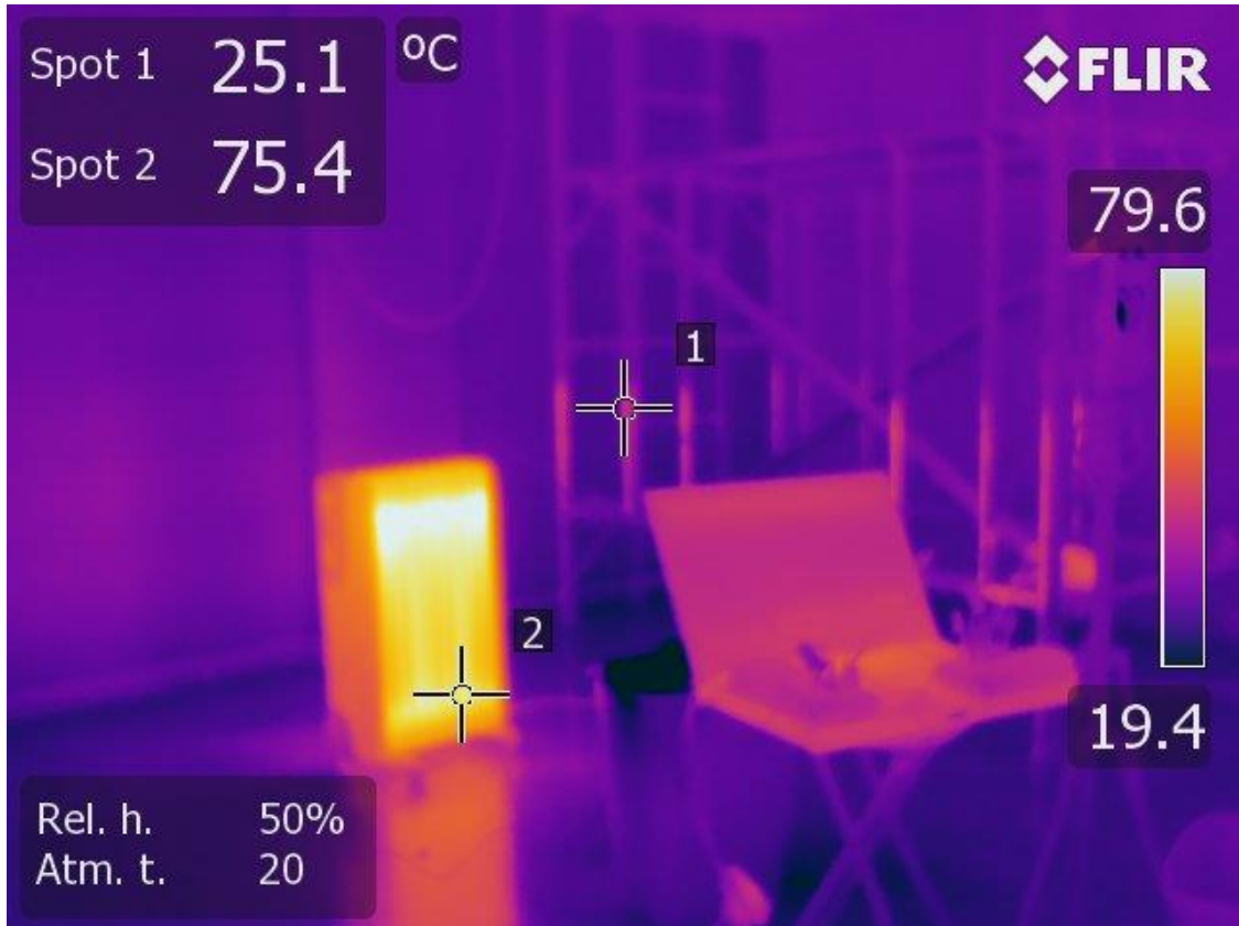
Figure 5-10 - Thermal imaging test using a portable radiator
