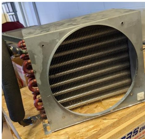
Figure 5-8 - Chiller heat exchanger submerged within the water tank
