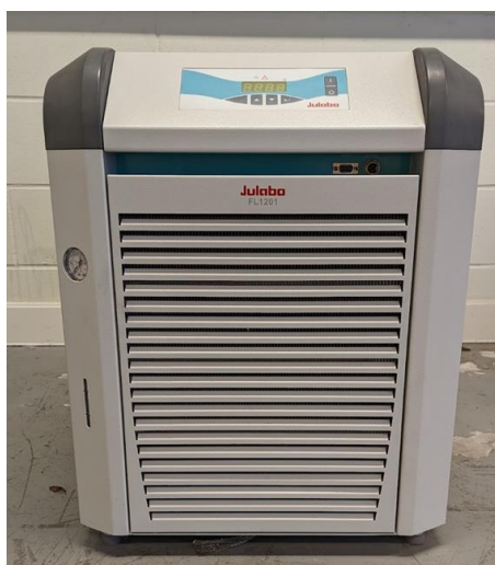
Figure 5-7 - Julabo recirculation chiller
