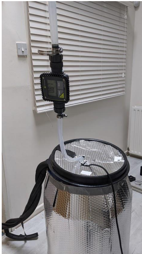
Figure 5-5 - Insulated water tank and digital flow meter
