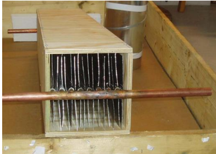
Figure 2-19 - Fins soldered to copper pipe surface in the heat exchanger (Davidsson et al., 2013)
