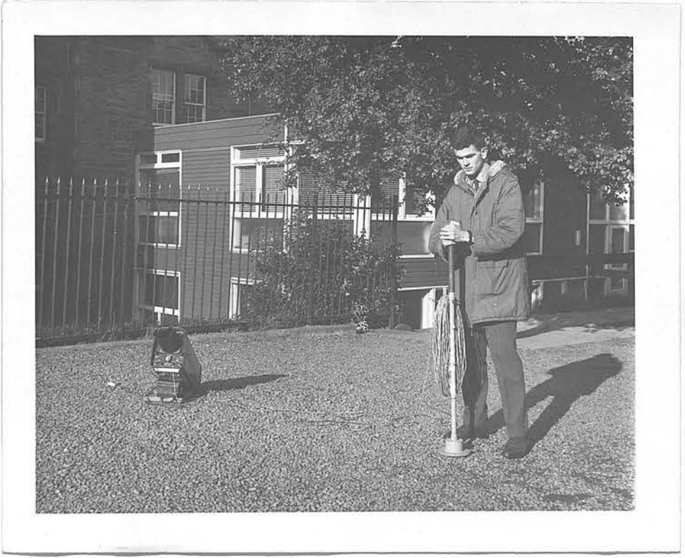
Plate 1: The 'Terra-Scout' portable refraction seismograph set up ready for use.
