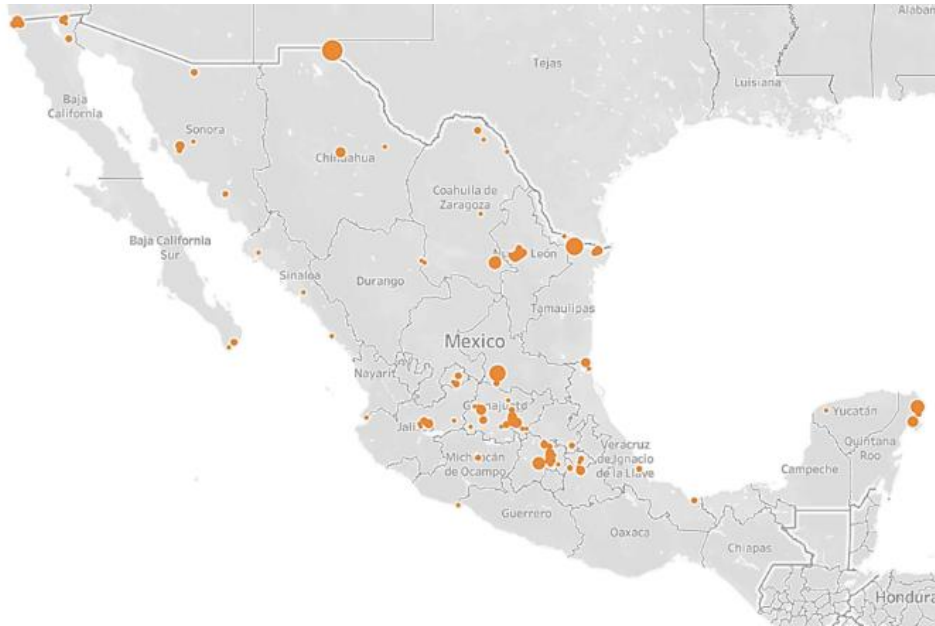
Figure 29 Distributed Generation Installed Capacity. Size of the balloons represents the size of the Installation. (Own elaboration, data SENER)
