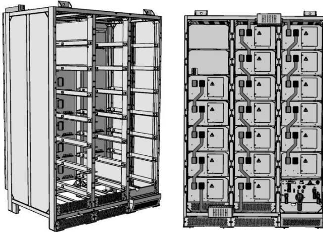
Figure 24 Empty Battery rack (left) and full rack (right) with battery modules. (Huawei, 2023)
