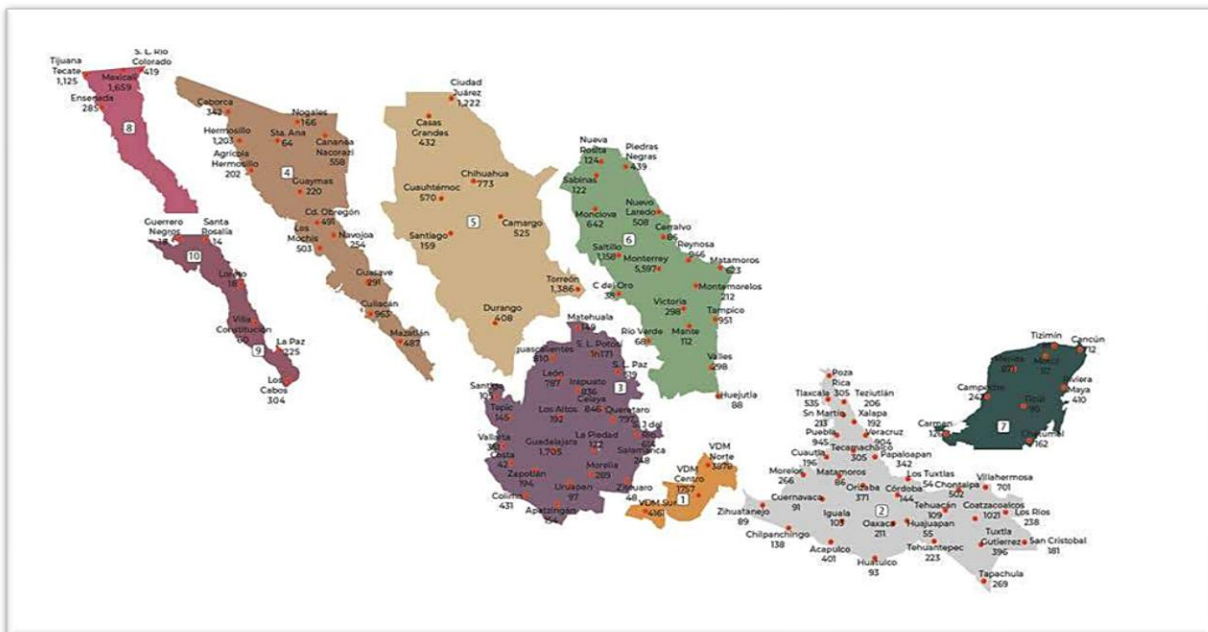
Figure 19 Max demand in 2023 registered for each node in the MEN for each Control Region. (SENER, 2023)
