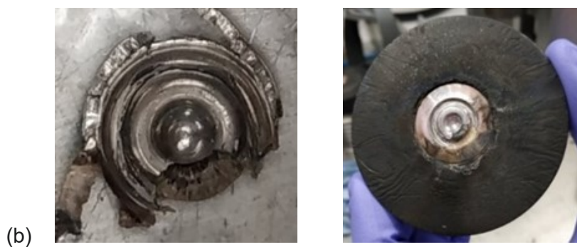
Figure 3.10 (a) Sequence of NPD patterns (rigid body refinements) obtained for perdeuterated 3,4,5-TNP over the pressure range of 0.1-4.5 GPa (b) Damaged ZTA anvil and Ti-Zr gasket
