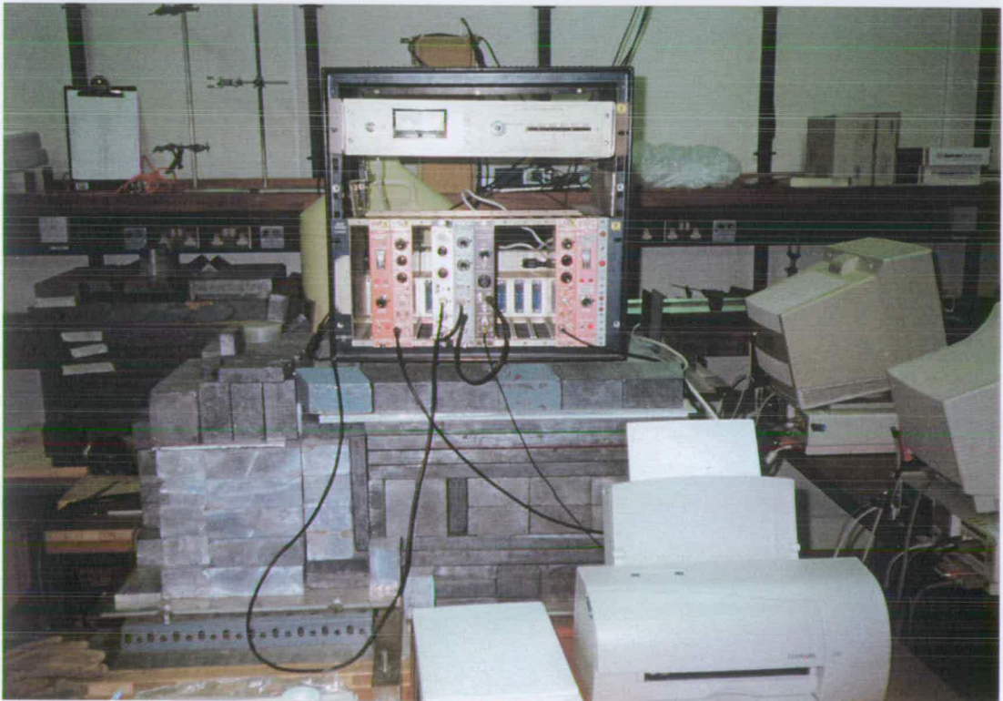
Figure 2.18. The set up for Ge-detectors. (a) Shows the detectors inside the lead shields. NGC is on the left hand side and REGe together with NaI (TI) are on the right side of the photo. (b) On the top of the shield the electronics for the detectors and on the right of the photo the PCs and on the front bench the printer is located.
