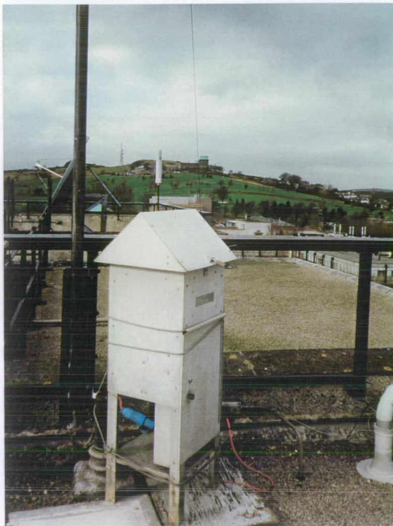
Figure 2.1. The high volume air sampler is located on the roof of JCMB.
