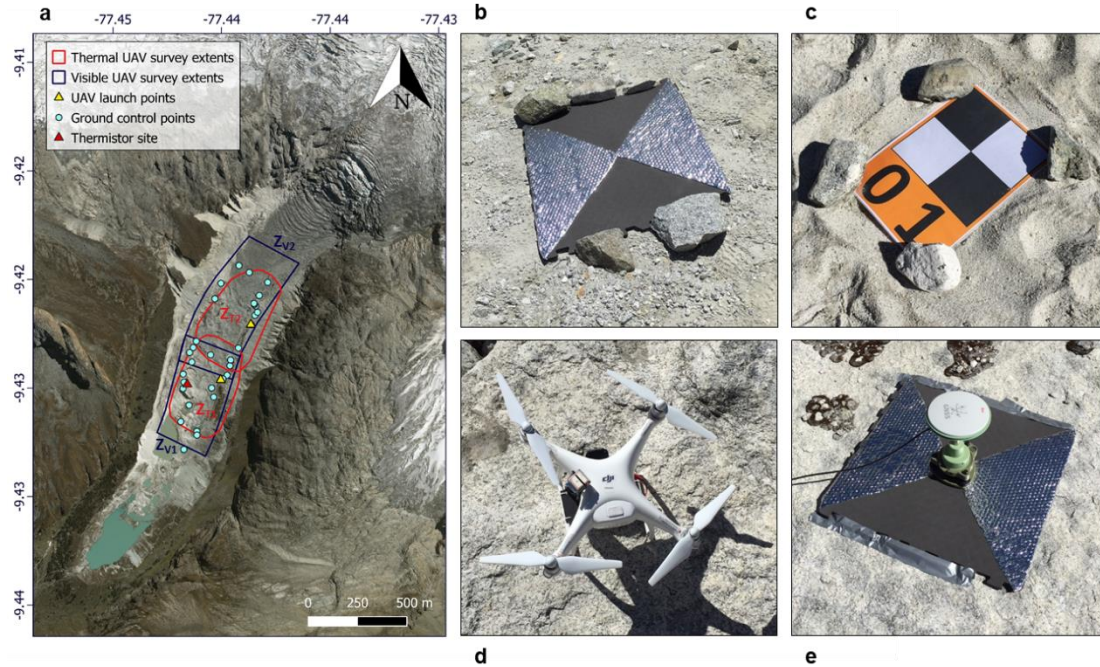
Figure 4.3. UAV survey setup at Llaca Glacier. (a) Extents of the thermal and visible UAV surveys, and locations of the two UAV launch points ground control points where GNSS data were collected and site where thermistors were installed within the debris layer. (b) and (c) Photographs of the materials used as ground control points for the thermal and visible UAV surveys respectively. (d) The custom-built UAV that was used to collect thermal imagery. (e) GNSS antenna setup for measuring the GPS position of each ground control point.
