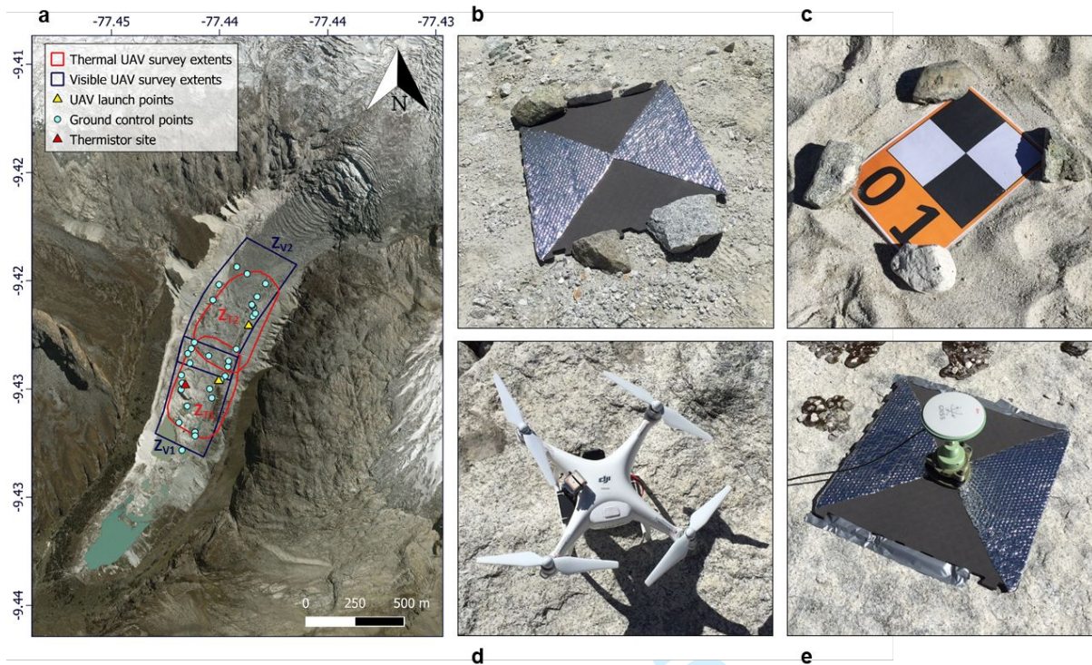
Figure 3. UAV survey setup at Llaca Glacier. (a) Extents of the thermal and visible UAV surveys, and locations of the two UAV launch points ground control points where GNSS data were collected and site where thermistors were installed within the debris layer. (b) and (c) Photographs of the materials used as ground control points for the thermal and visible UAV surveys respectively. (d) The custom-built UAV that was used to collect thermal imagery. (e) GNSS antenna setup for measuring the GPS position of each ground control point.
