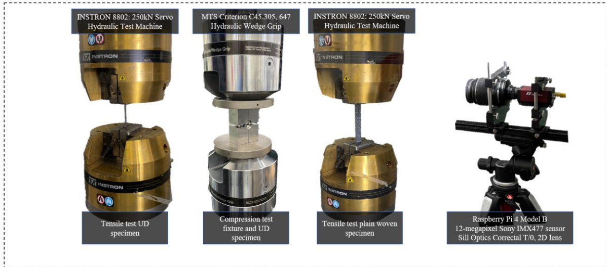
Fig. 3-2. Experimental setup in accordance with ASTM D3039/D3039M and D6641/D6641M for the UD and plain woven laminate.
