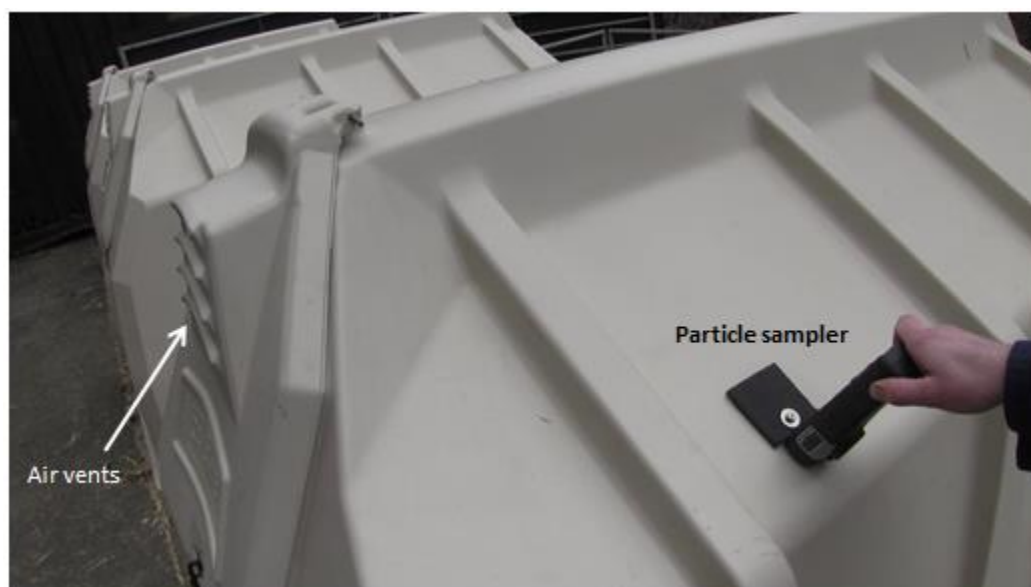
Figure 5.4 Placement of particle sampler in relation to rear air vents of hutch
