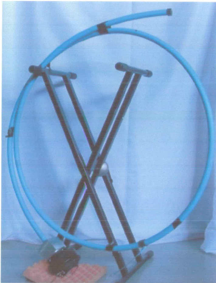
Figure 4.2: Photo of the APR source tube and loudspeaker
