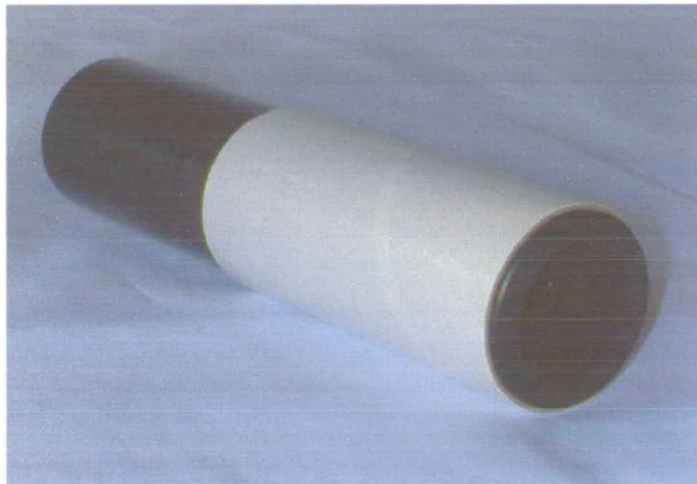
Figure 4.6: Schematic diagram and photo of mouthpiece for coupling with APR source tube
