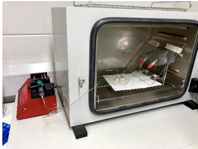
Figure 5.7: Image of first iteration of acrylic chip system (repeated from Figure 2.12 C). The image shows the chip sealed with glass cover slip inside the incubator, needles are attached at each inlet to the chip and inserted through septa into foil pouches containing media. The longer tube is connected to the chip outlet and a syringe which sits on the syringe pump outside of the incubator.
