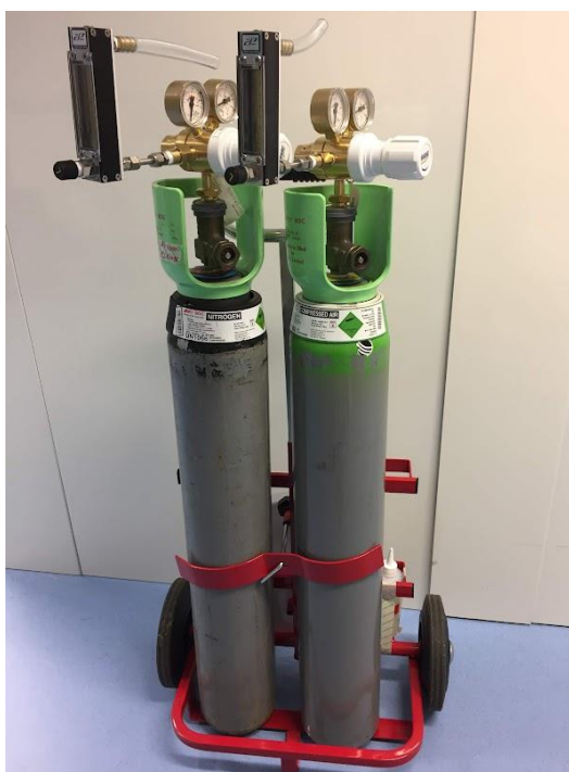
Figure 2.6: Image of compressed air and nitrogen gas cylinders with regulators and flowmeters in a portable trolley.
