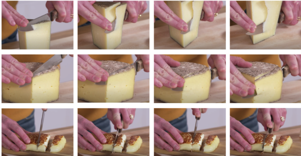
Figure 1.2: Various types of cheese and their cutting strategies. Firm cheeses, like Manchego, can be cut by simply pressing the blade downwards (top row). For cutting semi-soft cheeses, like Tomme, the deformations are compensated by applying a slicing-like movement (middle row). Softer cheeses with distinct viscoelastic properties, like Halloumi, are highly deformable and require dynamic adaptation of cutting movement for neat separation (bottom row). Screenshots from [6].
