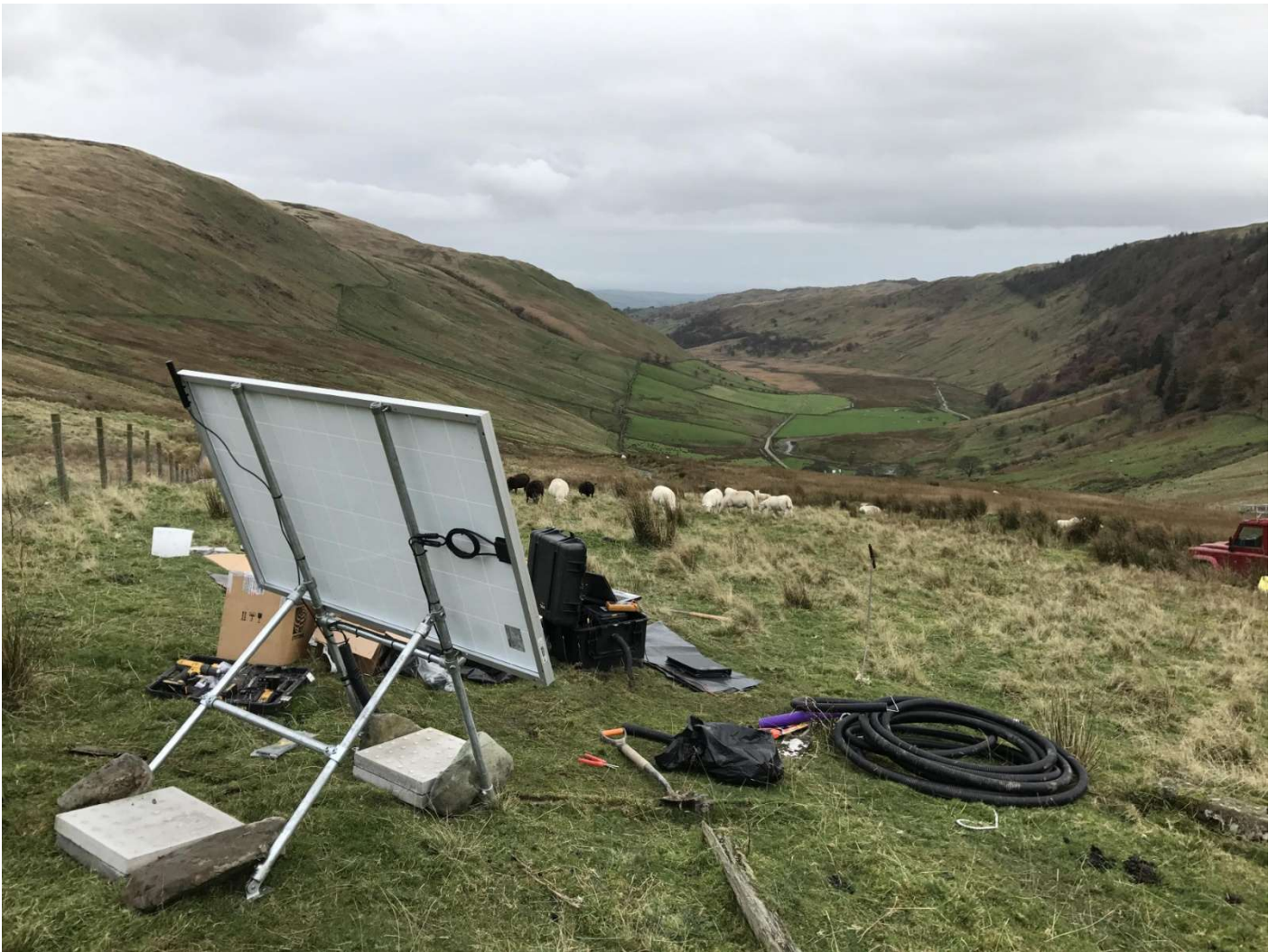
An earthquake monitoring station setup, including the solar panel and surrounding equipment.
