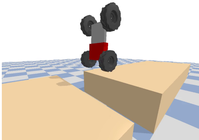
Figure 43: The wheeled jumping robot jumps across a gap. Please find the accompanying video at https://youtu.be/j2sIWL8m2pQ
