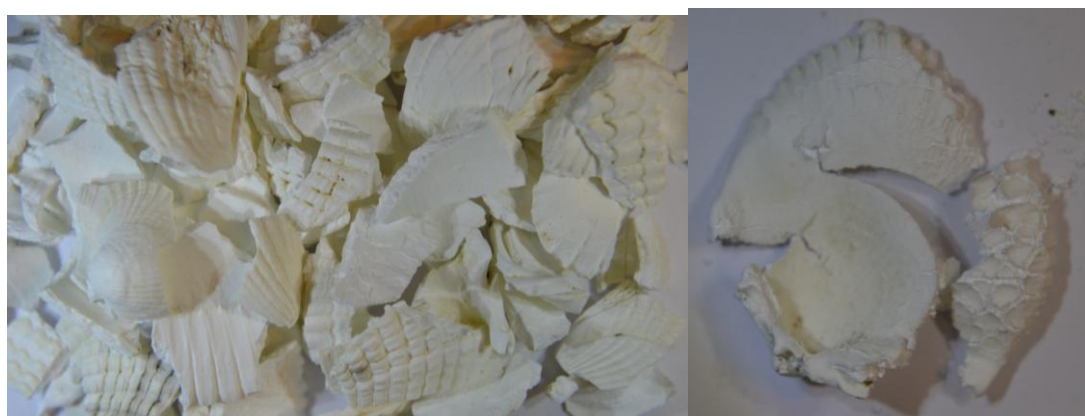
Figure 2.9 - BWC 950 – Shattered and whole C. edule valves heated to 950°C.
