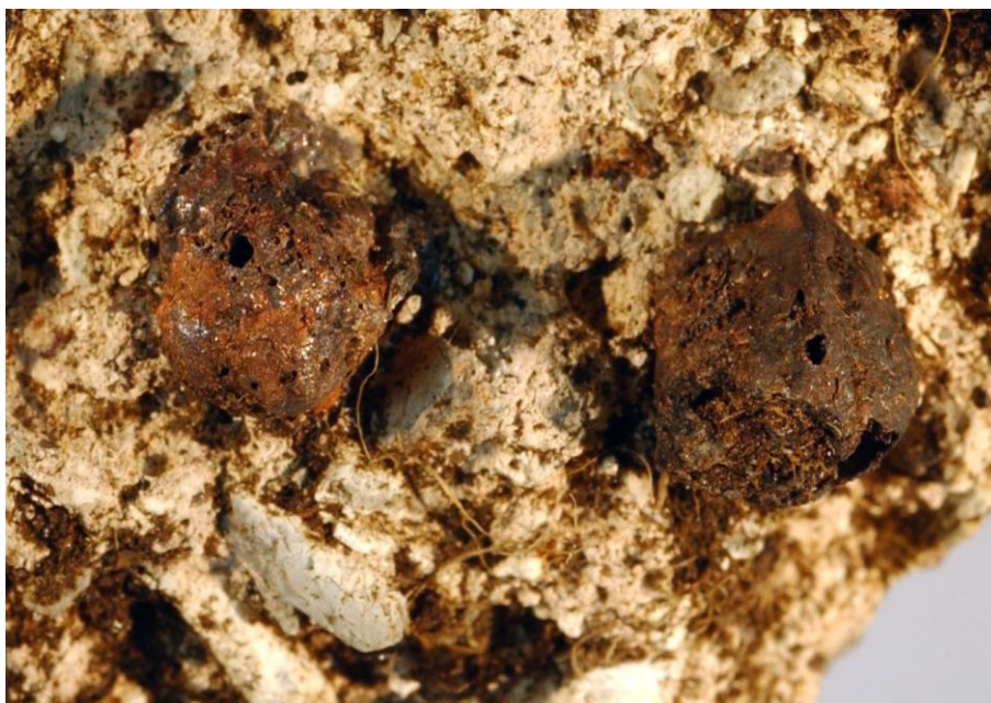
Figure 2.45 (above) - Vitreous inclusions within mortar of Teampull Ronain , North Rona. Field of view approximately 35mm.
