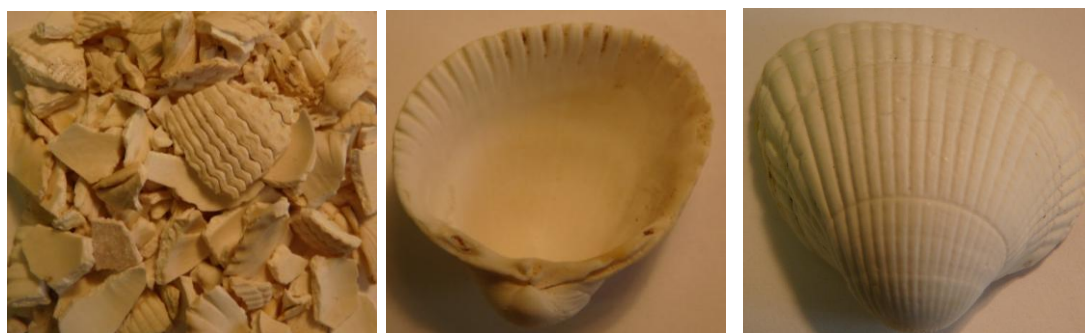
Figure 2.2 - BWC 150 – Shattered and whole C. edule valves heated to 150°C.
