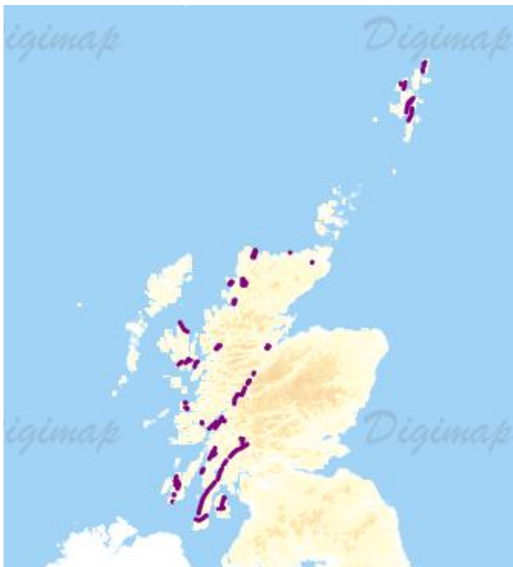
Map 1.1.10 – Main distribution of limestone within the survey area. After Scottish Lime Centre (2003, 11) with some added outcrops in Skye and Caithness. Where applicable local outcrops are plotted in more detail in volume III case studies.
