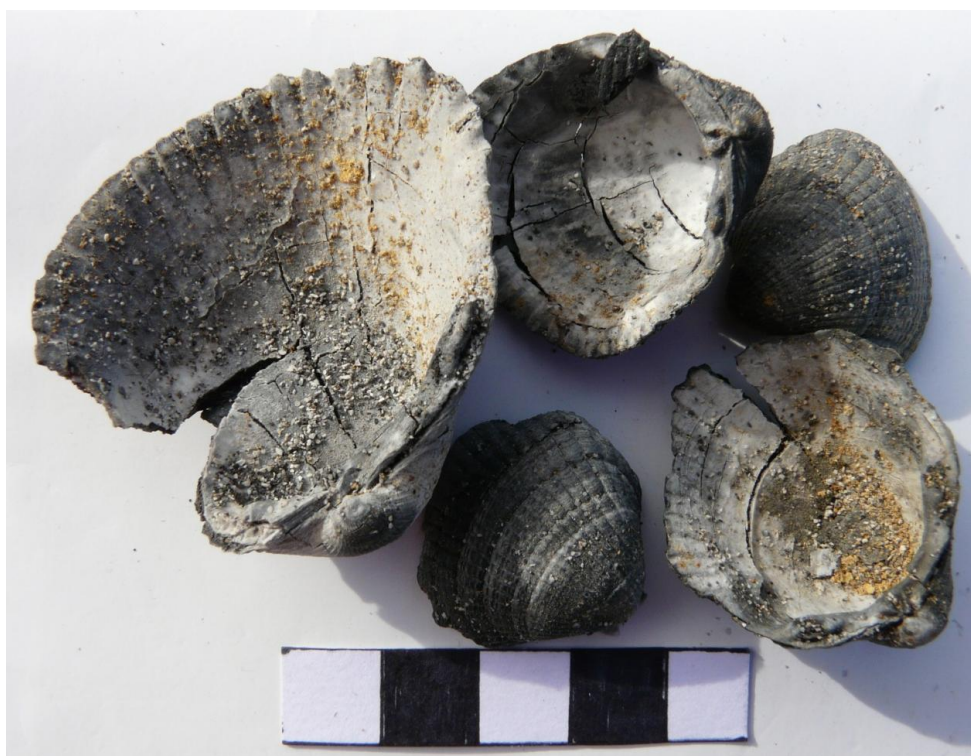
Figure 2.27 (above) - C. edule kiln-relicts from public demonstration and experimental shell-lime burn in replica 19 th -century kiln, Barra.
