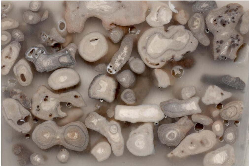
Figure 3.8 (above) - DVC.350 – Thick-section of maerl heated to 350°C.
