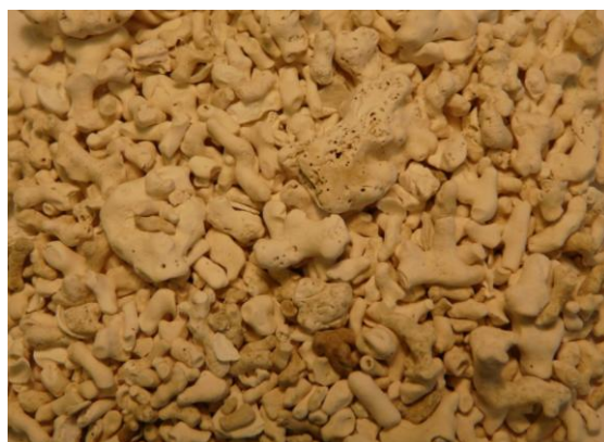
Fig. 3.7 - DVC.750 – maerl heated to 750°C.
