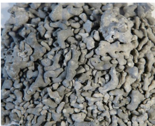
Fig. 3.5 - DVC.550 – maerl heated to 550°C.
