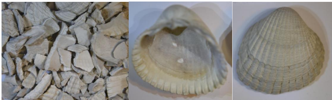
Figure 2.4 - BWC 000 – Shattered and whole C. edule valves heated to 400°C.
