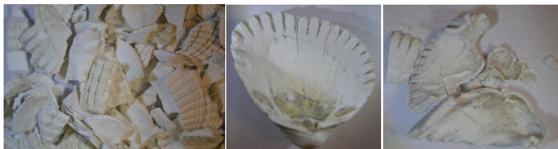
Figure 2.8 - BWC 750 – Shattered and whole C. edule valves heated to 750°C.
