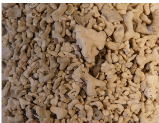
Fig. 3.6 - DVC.650 – maerl heated to 650°C.
