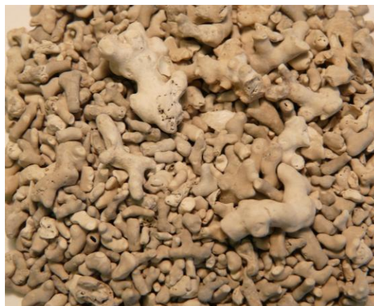
Fig. 3.3 - DVC.350 – maerl heated to 350°C.
