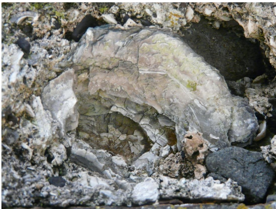
Figure 2.36 (above) – Heated O. edulis shell kiln-relict in mortar of Mingary castle N. range.
