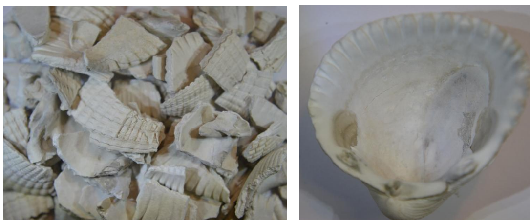
Figure 2.3 - BWC 350 – Shattered and whole C. edule valves heated to 350°C.
