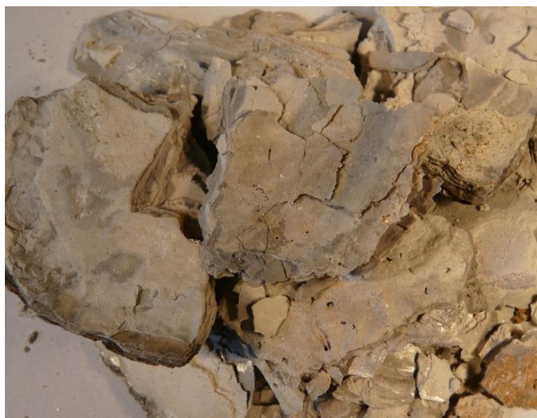
Fig. 2.29 - MDO.450; O. edulis shell heated to 450°C for 23 hours.
