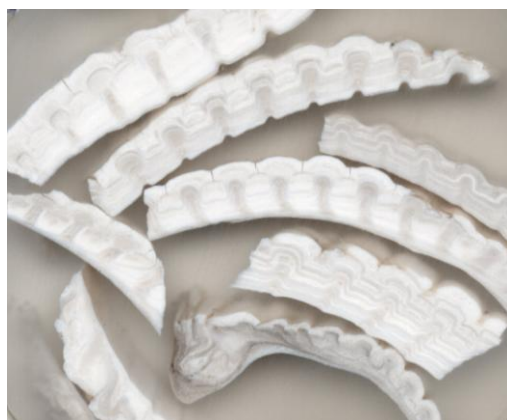
Figures.2.12 & 2.13 (above) - BWC.350 – Thick & thin-section; C. edule shell heated to 350°C.
