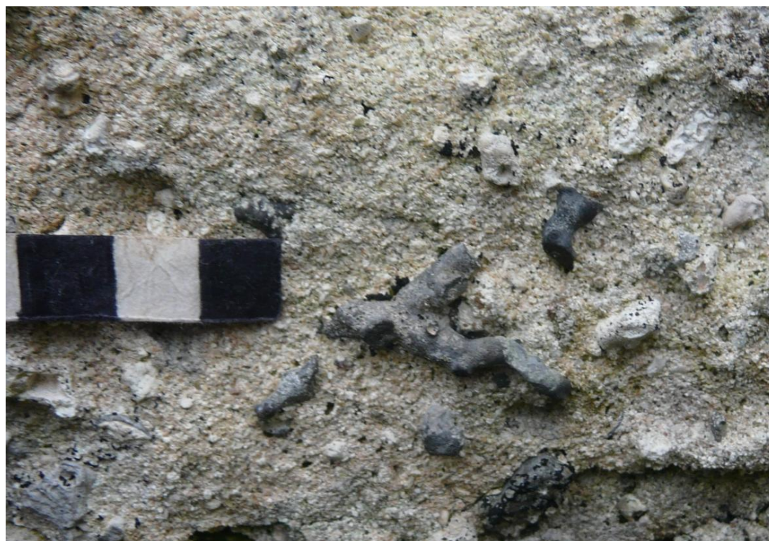
Figure 3.17 (above) – Range of altered maerl clasts in primary coating at St Mary's, Wyre, Orkney (Scale 10mm; photograph M. Thacker).
