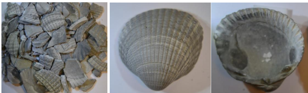
Figure 2.5 - BWC 500 – Shattered and whole C. edule valves heated to 500°C.
