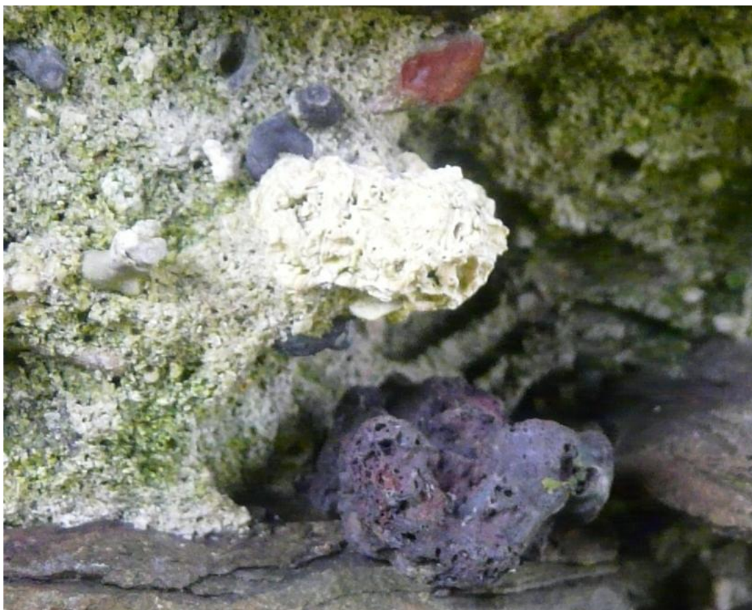
Figure 3.19 (above) – Range of altered maerl clasts in primary bedding mortar at St Mary's, Wyre, Orkney. Field of view approx. 60mm; photograph M. Thacker.
