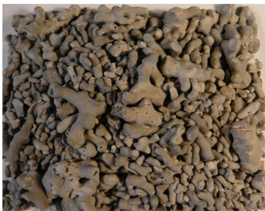
Fig. 3.4 - DVC.450 – maerl heated to 450°C.
