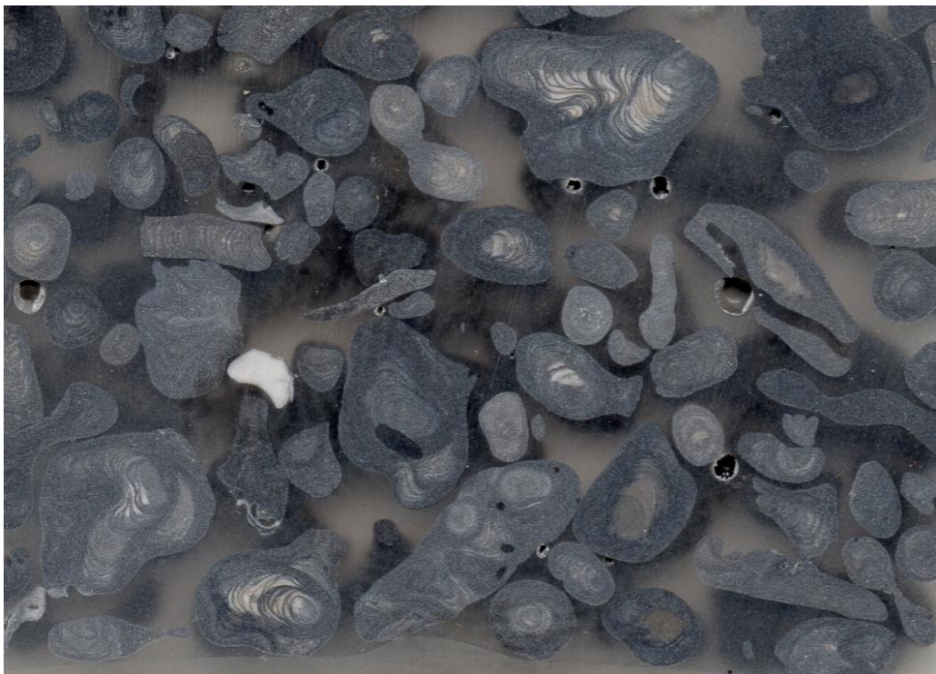
Figure 3.9 (above) - DVC.550 – Thick-section of maerl heated to 550°C.
