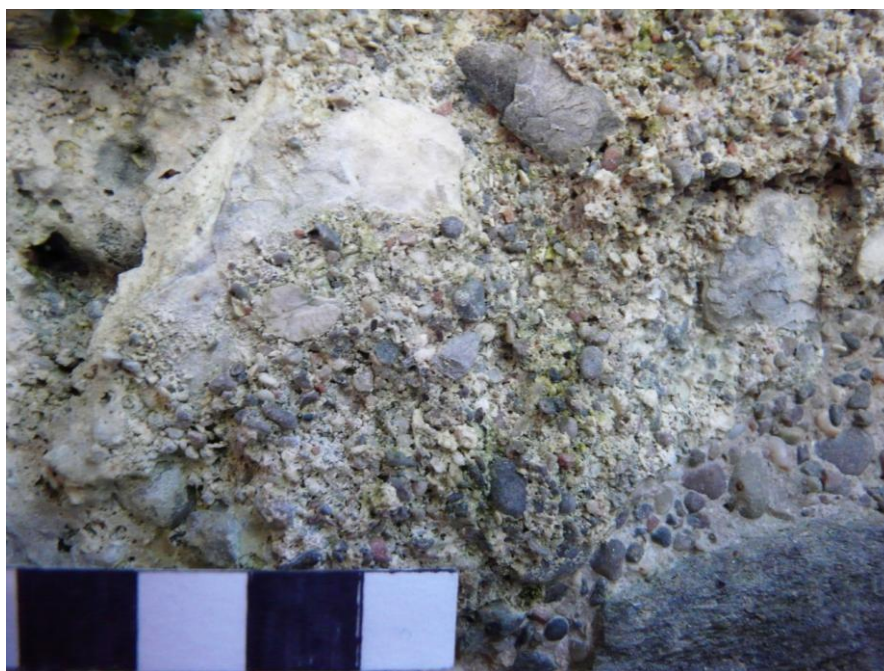
Figure 2.37 (above) – Range of heated O. edulis shell kiln-relicts in internal coating mortar of St Ronan's parish church, Iona. Scale 10mm.
