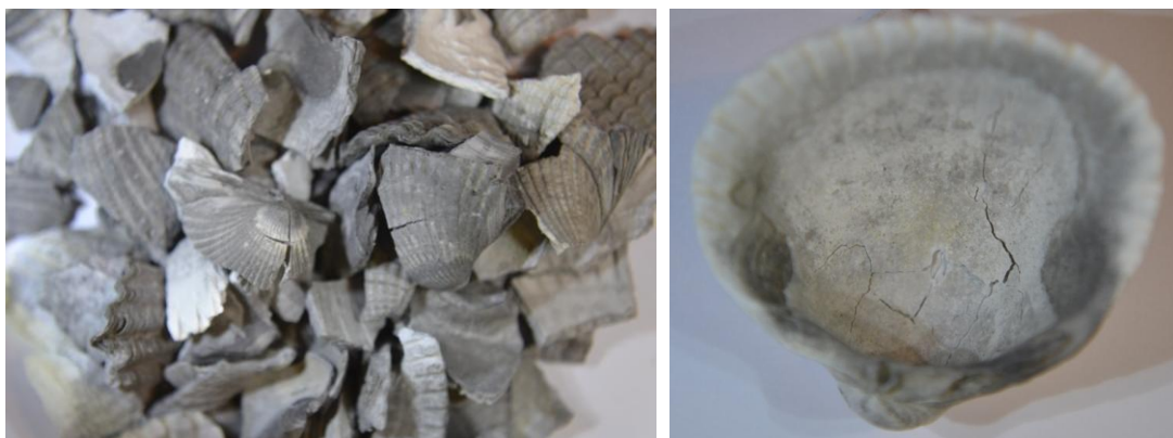
Figure 2.6 - BWC 550 – Shattered and whole C. edule valves heated to 550°C.
