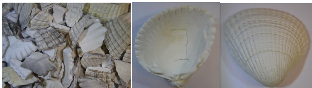
Figure 2.7 - BWC 600 – Shattered and whole C. edule valves heated to 600°C.
