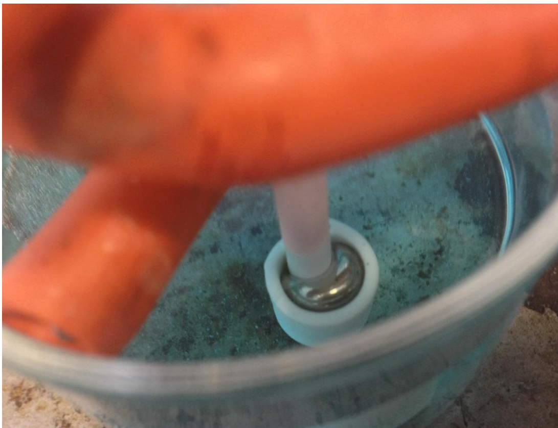
Figure 3.2: Image of the meniscus on the mercury macroelectrode used in this thesis.
