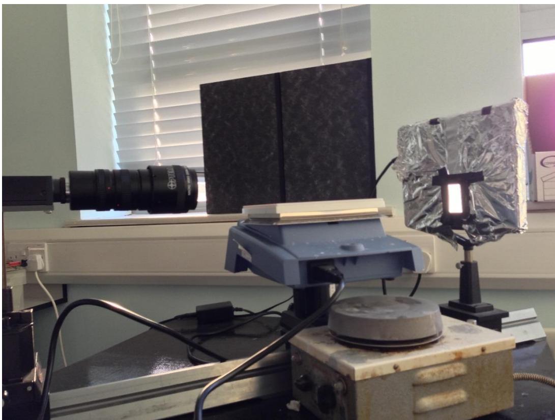
Figure 3.5: Goniometer stage replaced by a ceramic hotplate.
