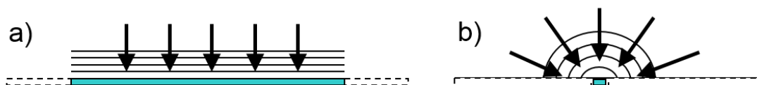
Figure 2.2: Comparison of diffusion at a) a macroelectrode and b) a microelectrode. The coloured areas represent the electrode area, the lines around the electrode represent the diffusion layers and the arrows indicate the diffusion path of ions towards the electrodes.
