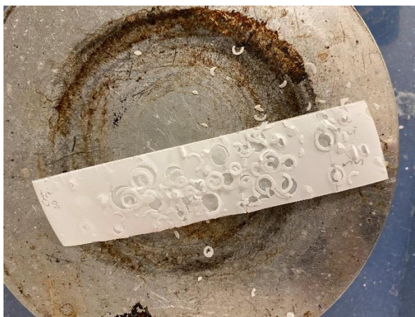
Figure A3. Insufficient drying and quick heating can lead to bubbling and destruction of silica coated layer.
