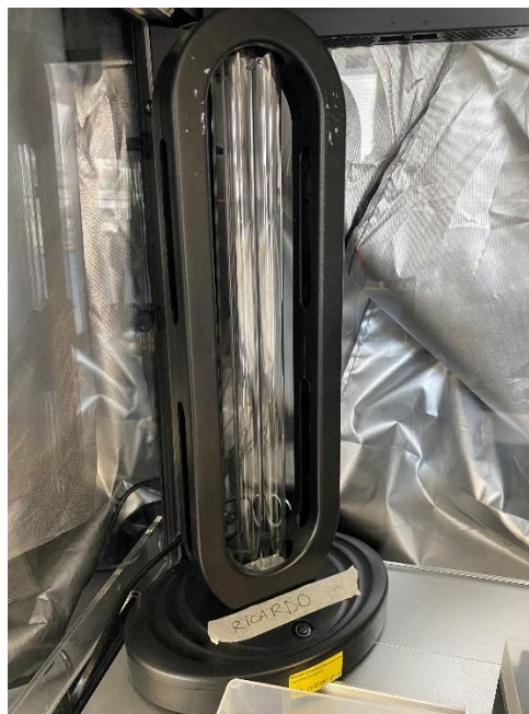
Figure 3.13. UV lamp located in a corner of the Opentrons robot. It can be operated via remote control. When the ON button is clicked, it takes 5 mins to start. On that time, alarm beeps to warn surrounding people about accidental exposition. The robot cover should be always used when operating the UV lamp.
