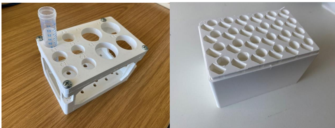
Figure 3.22. 3D printed racks used in Opentrons runs. The rack for 24 microtubes is provided by Opentrons, while the design on the left for 5ml and 15 ml Falcon tubes is an open-source design provided by Trevor Ho (github/tyhho).
