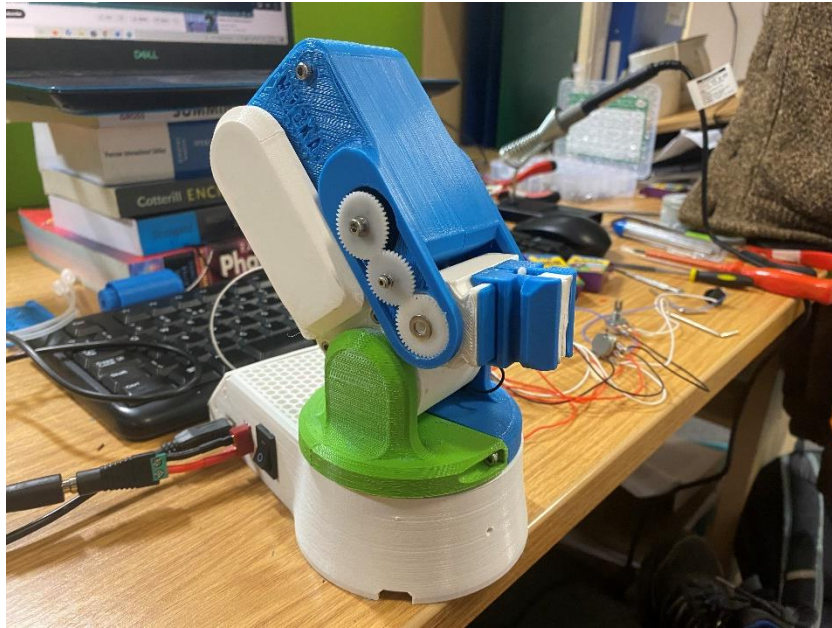
Figure 3.20. The fully assembled robotic arm. The external power plug and the switch is shown on the left side of the robot.
