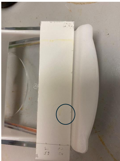
Figure A1. A TLC run of a Bacillus subtilis supernatant sample using a solvent mix of Chloroform: Methanol: Water 20:9:1. The shown plate was stained with iodine. The circle indicates the unique spot that was identified after the run.
