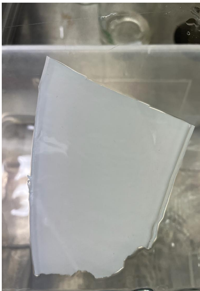
Figure 6.2: Cellulose acetate support fabricated using a polymer dope solution of CA, Cyrene™ and methanol (50:50) using water as the non-solvent
