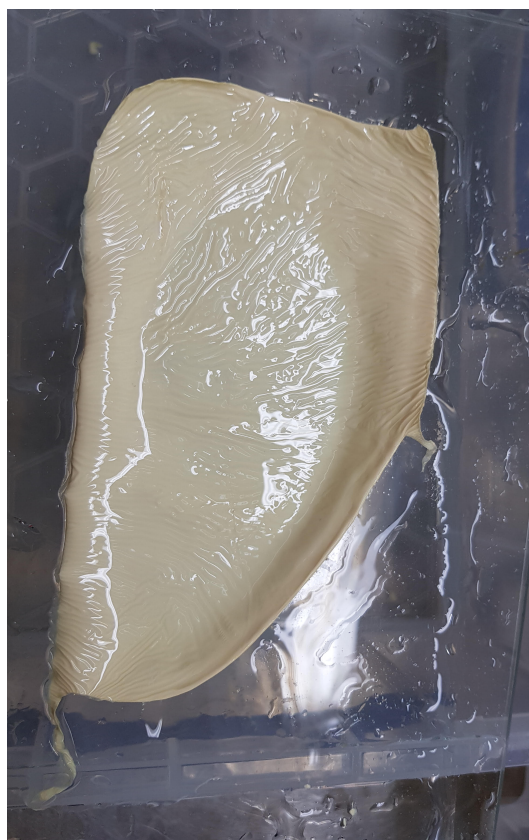
Figure 4.3: Support cast using a PI and 50:50 NMP and Cyrene™ dope solution using DI water as the non-solvent, the casting and coagulation took place at room temperature
