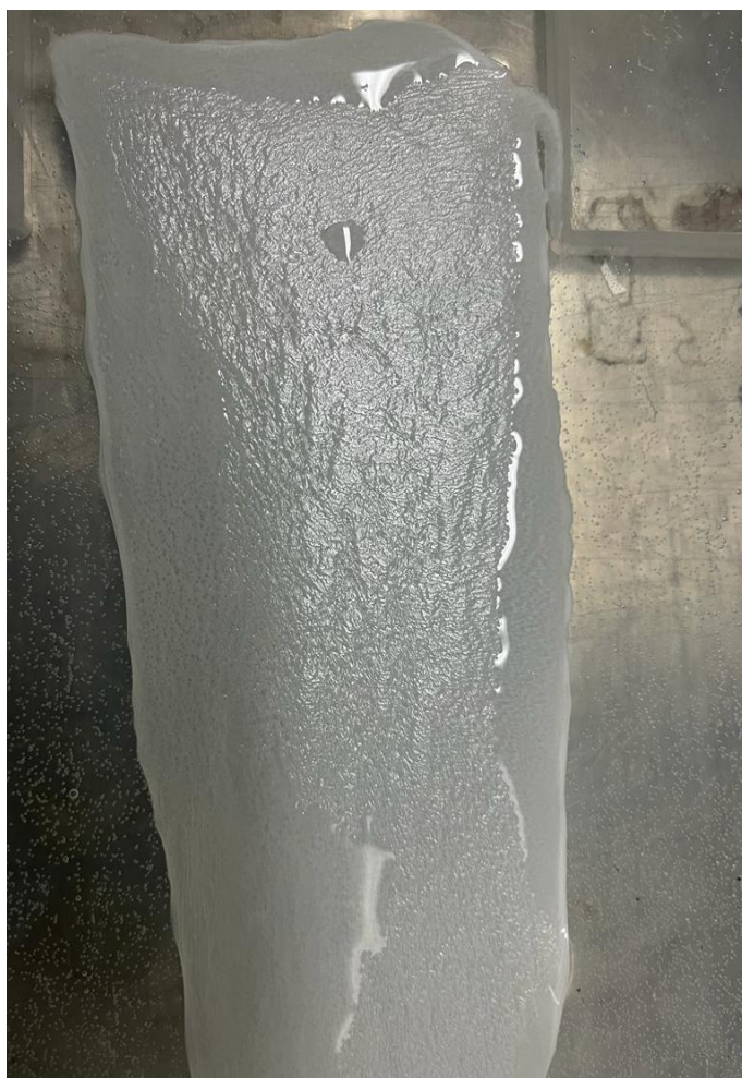
Figure 6.1: Cellulose acetate support fabricated using a polymer dope solution of CA, Cyrene TM and acetone (50:50) using water as the non-solvent
