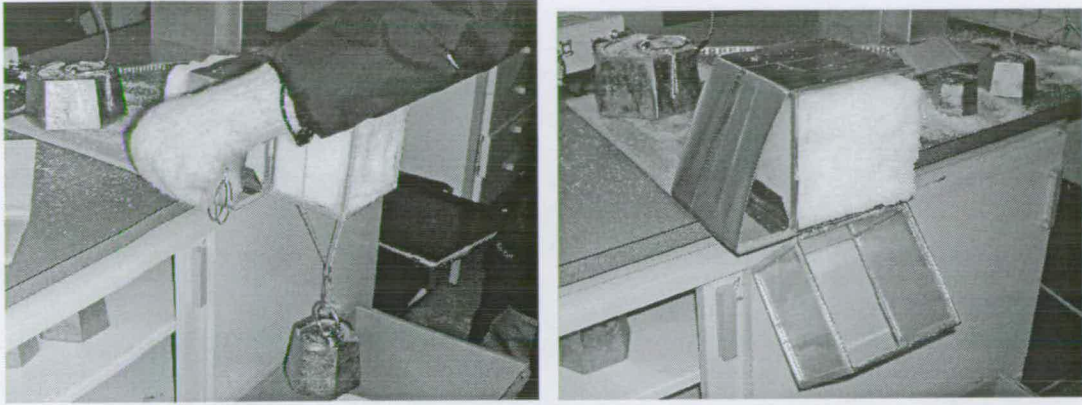
Figure 6.4: The mode I experiment. Left; Cutting through the snow block at the gap between the box sections with a wire. Right; The device and fracture surface after failure. Although not apparent in this image, the fracture surface is rough, easily distinguishable from the surface caused by the cutting with the wire.
