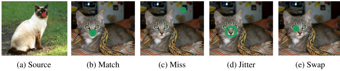
Figure 2.2. For the keypoint denoted in red in the source image (a), we see the correct match in (b). If the point matches with the background it is a miss (c), if it is close to the correct location it is a jitter (d). If the match is in the correct vicinity but closer to another semantic part, it is a swap error (e).
