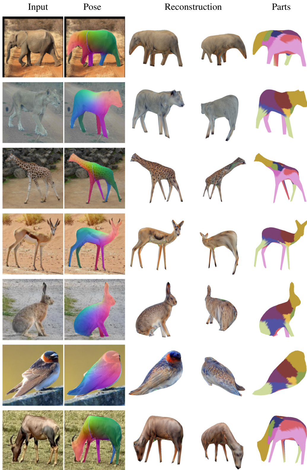
Figure 3.7. SAOR capable of predicting the 3D shape of an articulated object category from a single image. Our model is trained on multiple categories simultaneously using self-supervision on single-view image collections. It can efficiently predict object pose, 3D shape reconstruction, and unsupervised part-level assignment using only a single forward pass per image at test time in a category-agnostic way.
