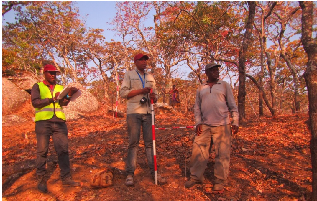
Figure 1. Site-based plot measurements-Ntchisi Forest-2019; (Top)-Crown diameter measurements taken from the long and short axes of the crown intersected at 90^{\circ} , and (Bottom) – Verification of horizontal distance from plot-centre to tree using a linear tape.
