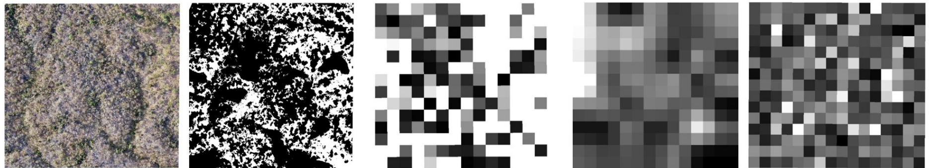
Figure 65. Comparison of Crown Distribution measured at 50ha in P2; (Left – Right): (i) UAV Orthophoto-7cm pixel spatial resolution, 0-255 scale; (ii) FC-7cm pixel spatial resolution, 0-100% scale; (iii) DTM -50m pixel spatial resolution, 634-708 scale; (iv) CHM -50m pixel spatial resolution, 0-55m scale; and (v) Sentinel-1-C -50m pixel spatial resolution, 0 to -0.6 decibels scale.
