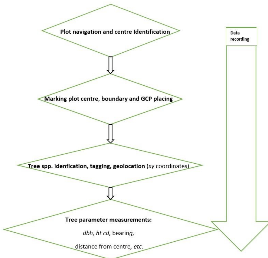
Figure 16. Top-Bottom: Schematic representation of key tasks undertaken, and parameters measured during ground-based inventory in Ntchisi Forest-2019.
