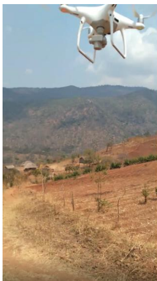
Fig. 2. Left-UAV (DJI-Phantom-4 Pro+ quadcopter) with camera sensor mounted on a gimbal, set at nadir angle of acquisition, vertically taking-off to Msankhire plot (P3) flight mission in Ntchisi Mountain Forest; Right-Structure from Motion (SfM) Photogrammetry technique
