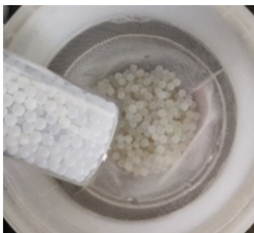
Figure 3.7: Colour difference between pristine, unused beads, and those which had been used in testing multiple times
