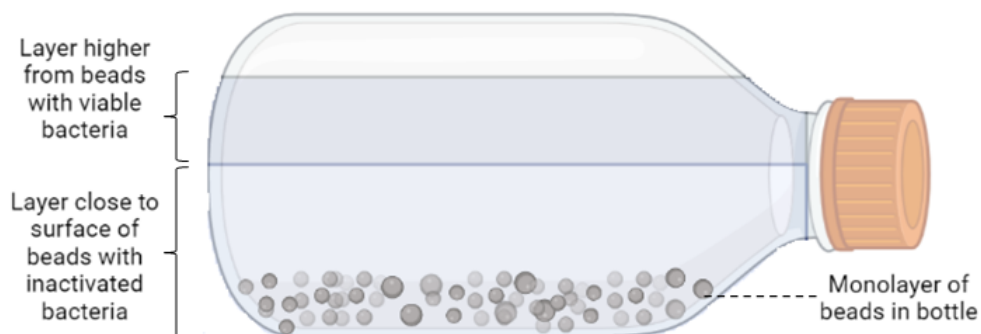
Figure 3.4: Mass transport schematic, illustrating how two layers of water may form close to and far away from the catalyst layer.
