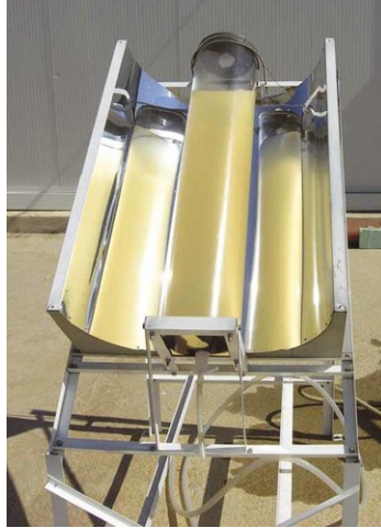
Figure 1.1: Image from study by Ubomba 46 on the implementation of a CPC with a 25 L methacrylate tube for enhanced SODIS, presented with permission from John Wiley and Sons Publishing.
