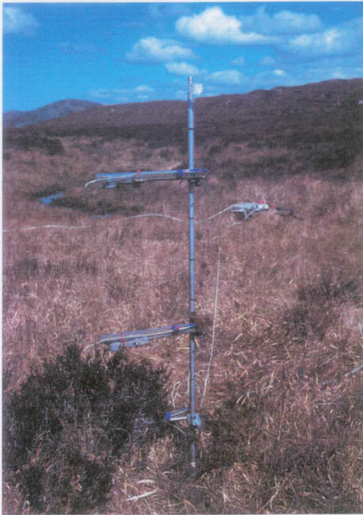
Figure 4.1. Plots on site A prior to burning, showing the retort stand and glass tubing used to protect and support the thermocouple wires.
