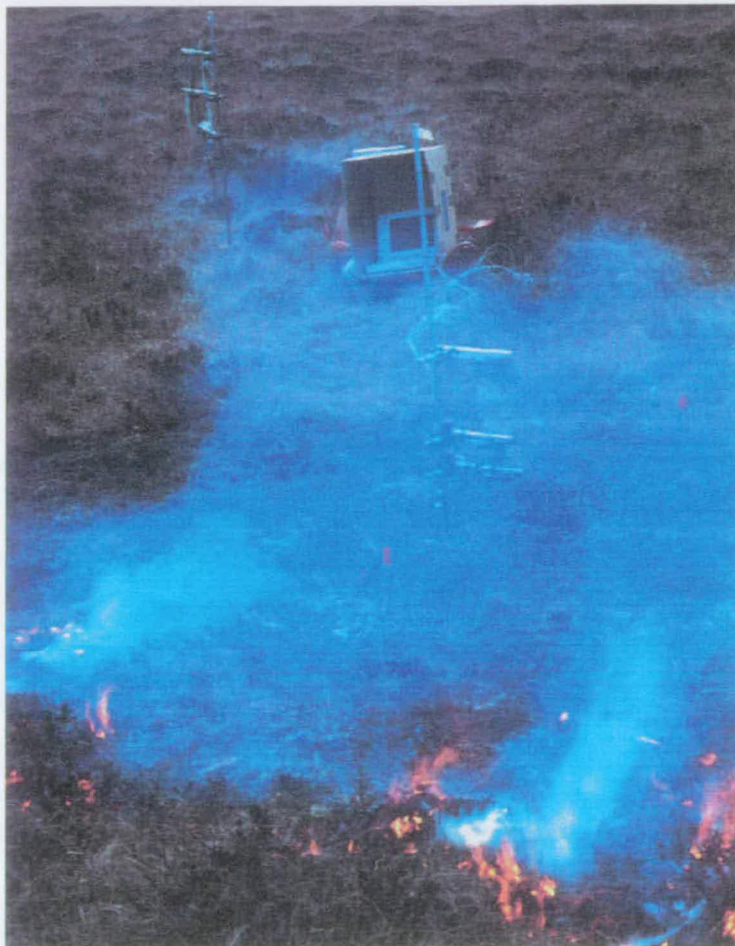
Figure 4.2. Fire going through a medium fuel plot (site C) on the first day of burning (18/4/98). Note the small flame height and the discontinuous nature of the fire-front.
