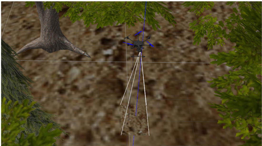
Figure 5.5: The biorobot's camera has a relatively narrow field of view and is downward facing.
