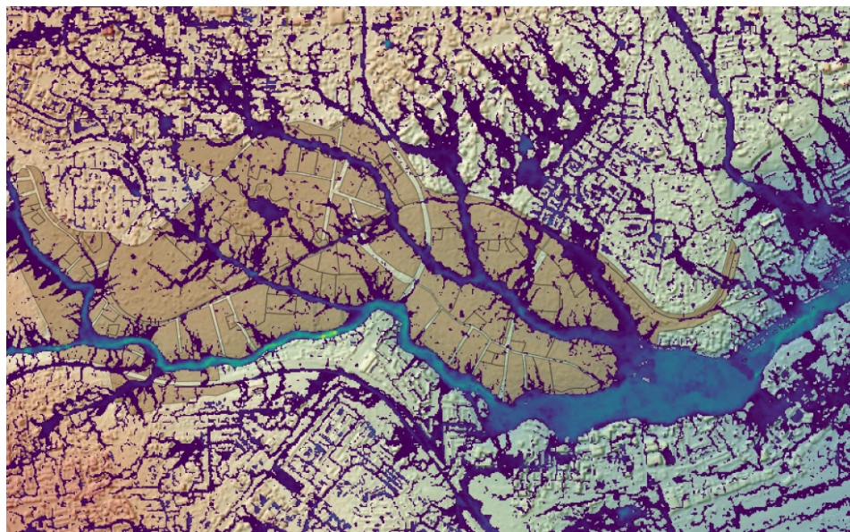
Flood event simulations that will later feed the calculation of impacts within each urban scenario.
