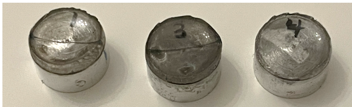
Figure 7.3 – Cryo-FIB/SEM specimens. All specimens are PDMS 80°C. Specimens 1 and 3 are cut with a scalpel, and specimen 4 was abraded. Specimens 3 and 4 have been platinum coated and imaged.
