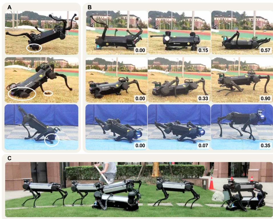
Figure 4.1: Challenging locomotion scenarios and agile maneuvers of a quadruped robot. (A) Three challenging scenarios of the Jueying robot during various tests: unexpected body contacts with the environment and unpredictable robot states. The white circled regions highlight unusual contact that can occur at any part of the body. (B) Different adaptive behaviors from our proposed learning framework that generated dynamic motions and complex coordination of legs for immediate recovery from failures. Time in snapshots is measured in seconds. (C) Resilient locomotion using adaptive skills in the presence of unexpected disturbances.
