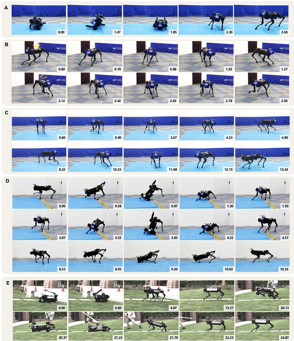
Figure 4.5: Dynamically synthesised MELA policy running on a real quadruped robot and demonstrating adaptive and agile locomotion behaviours. (A) Successful fall recovery performed by the MELA expert, inheriting original skills from the pre-trained experts. (B) Newly emerged skills, dynamic steering on the spot, naturally learned through the MELA framework. (C) Target-following experiment with simultaneous trotting and steering using online synthesised skills. (D) Target-following experiment showing the capability of failure-resilient trotting and critical recovery within one second (averagely 0.5 second for restoring body posture and 0.4 seconds for returning to the trotting mode). (E) Adaptive trotting and fall recovery experiment on a sloped grass field, showing the capability of robust traversal in unstructured environments. (Time in snapshots is in second).
