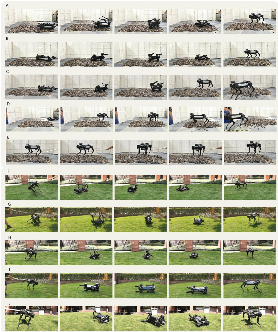
Fig. S11. Adaptive and agile locomotion behaviours on pebbles and grass demonstrated by MELA policy. (A-E) Self-righting and trotting on pebbles. (F-J) Self-righting, trotting, and adaptive fall recovery in presence of various pushes on grass.
