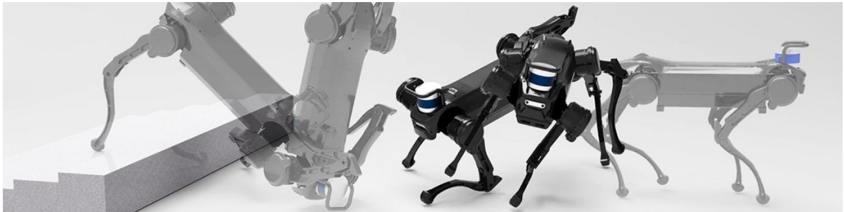
Figure 1.3: Fall-resilient locomotion on Jueying using proposed Multi-Expert Learning Architecture (MELA).
