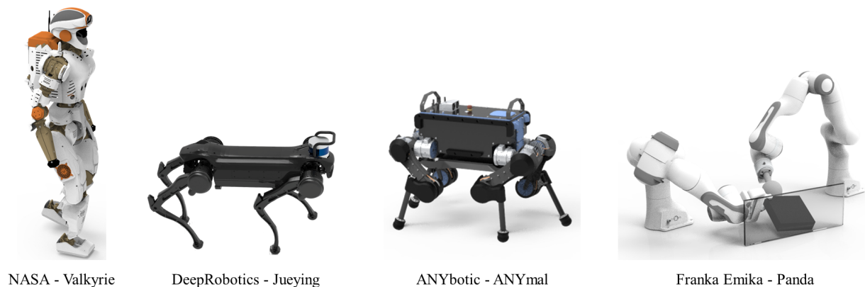
Figure 1.1: Robots on which the algorithms of this thesis were applied on: humanoid Valkyrie, quadrupeds Jueying and ANYmal, and dual arm manipulators Panda.
