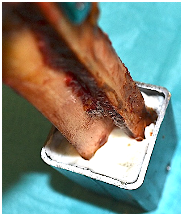
Figure 4.8: Proximal fixation with PMMA cement pot (view from underneath).
