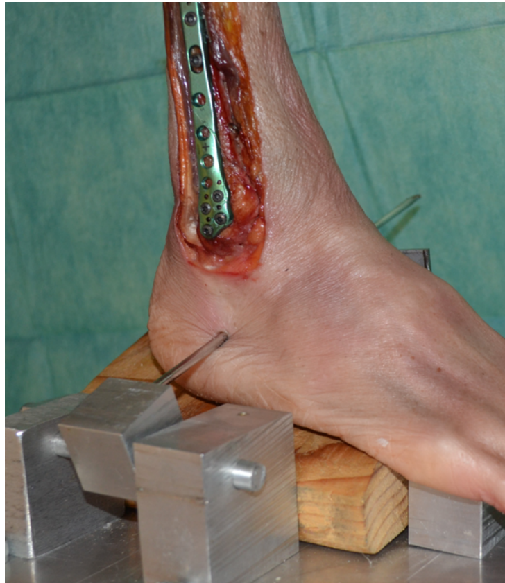
Figure 4.5: Distal transcalcaneal fixation secured into custom-made 20° baseplate.
