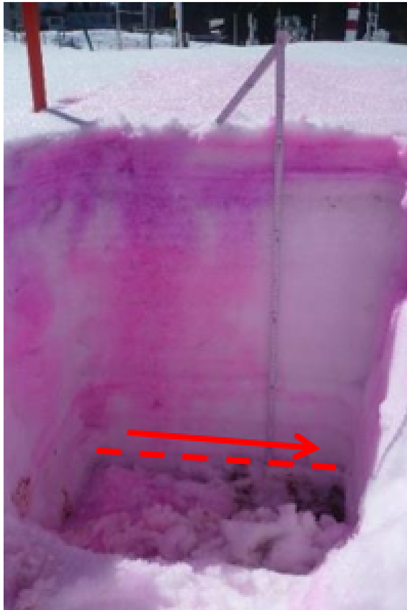
Figure 4.7: Dye tracing experiment carried out on 20th March 2019. The density contrast, along which horizontal flow occurred, is marked.
