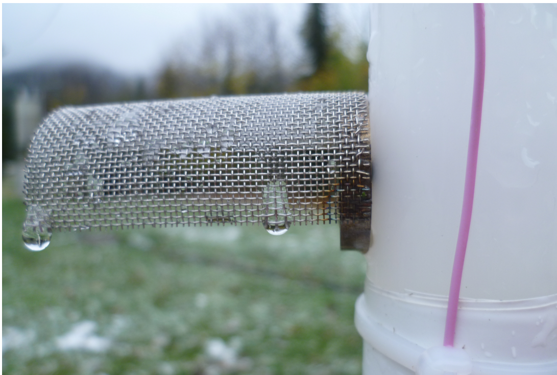
Figure 3.9: Close-up photograph of mesh ERT electrode during installation in November 2019
