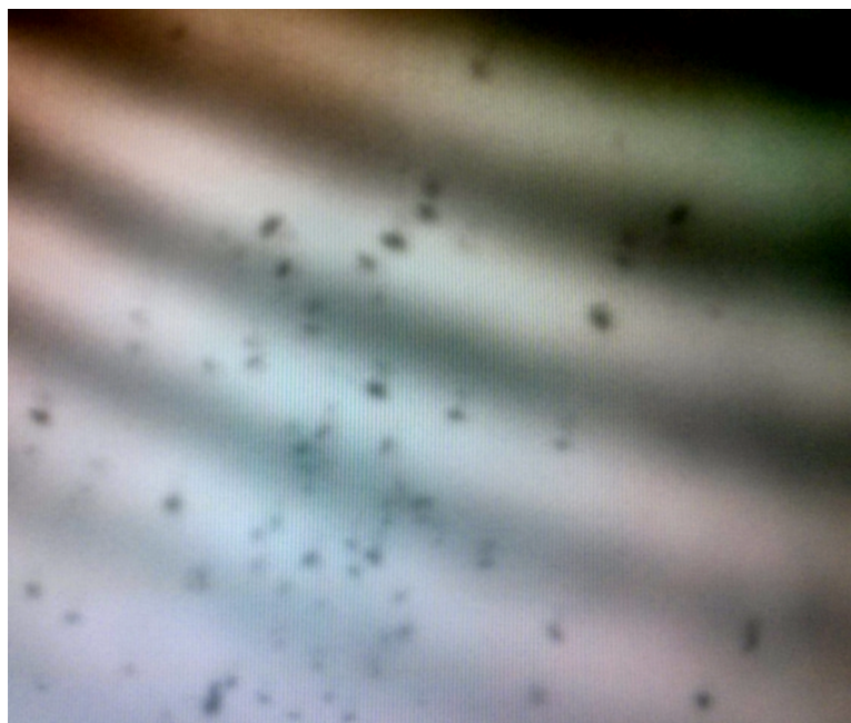
Figure 3.12: Example of light and dark interference fringes produced by the phase shift between the reference light signal and the reflectance from the sample surface.
