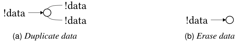
Figure 3.7: Illustrative diagrams of resource actions duplicating and erasing a copyable resource atom
